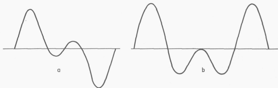
Fig. 16. The influence of the phase relation between the first and the second harmonic at the shape of the oscillogram, if the exit slit is adjusted near the central maximum of the diffraction pattern. The phase difference between the first and the second harmonic is: a. 0^\circ ; b. 45^\circ . The amplitude of both harmonics have been taken equal to each other.
