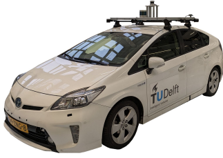
(a) The demonstrator vehicle and its roof-mounted sensors.
