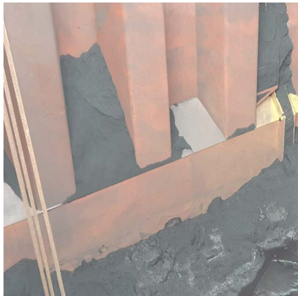
Figure 2.13: Stagnant zone in a bulk carrier hold
