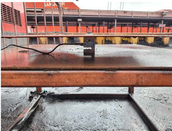
(b) Load cell mounted between a table and a plate
