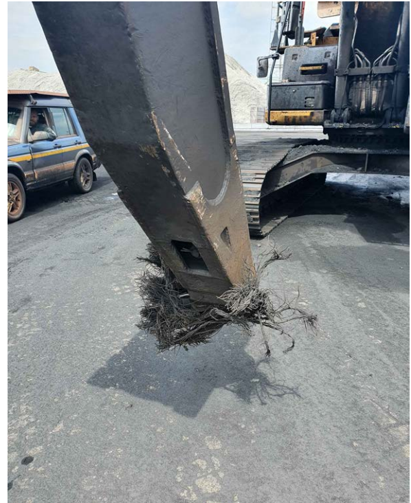
(b) Closeup of the damaged brush
