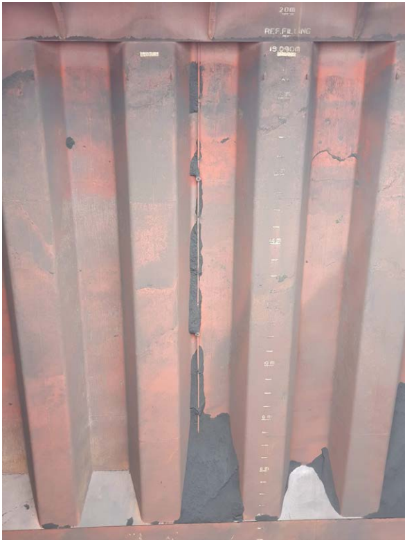
(c) Stuck coal behind a sounding pipe in a transverse bulkhead
