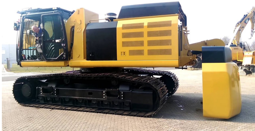
Figure 5.4: Removal of the counterweight on an excavator [101]
