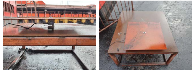
(c) Load cell mounted between a table and a plate (d) Table with the force measuring plate
