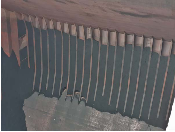
(a) Side shell frames full of coal
