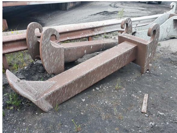
(b) A scraper with a different shape but the same width
