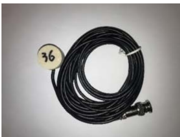
Figure 3. Photo of a Smart Aggregate (SA).
