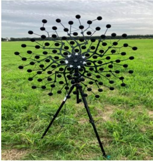
Figure 22: The array test setup during the experiments
