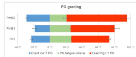
Bit1 is 35/50 pen bitumen, PmB1 is standard PmB, PmB2 is highly modified PmB
