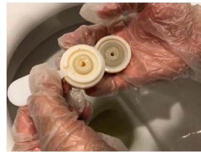
Fig. 12. Outcome of the third iteration: filter holder design
