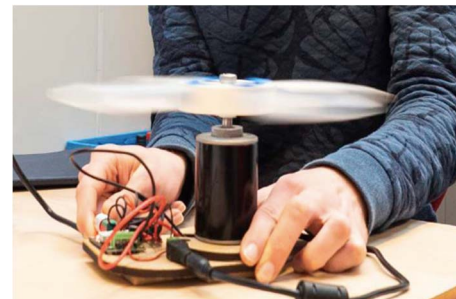
Fig. 13. Low-cost, locally manufacturable and maintainable centrifuge
