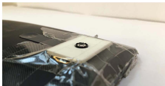
Fig. 4. Reverse phone objective lens added to the camera module
