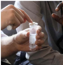
Fig. 7. 2 nd iterated design 3D-printed filter holder placed on urine cup
