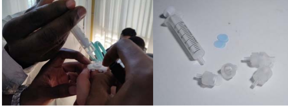
Fig. 10. The difficulty of using the customized holder (Left) and the standard filter and filter holder (right)
