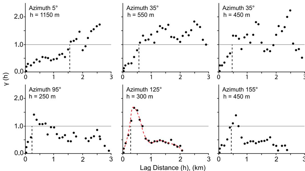
**Figure 10.** One-dimensional directional variograms for floodplain aggradation cycle H with different azimuths in the McCullough Peaks area (Wyoming, USA). Vertical dashed lines indicate the ranges along different azimuths. Red dashed line in the panel with azimuth 125° shows an example of a non-monotonic variogram that is different from traditional, monotonic ones (e.g., azimuth 5°). Information on how to read variograms is detailed in the Methodology section.
