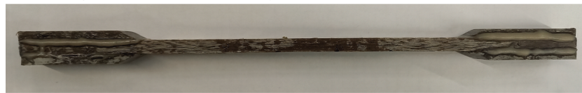
(b) Side view of a prepared sample of layup A with tapered composite end tabs
