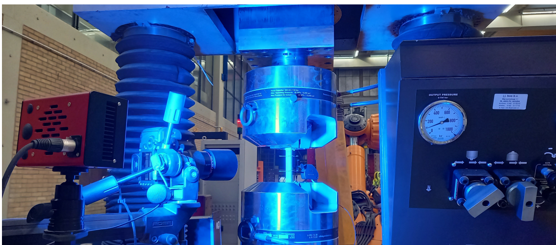
Figure E.1: Quasi-static tensile test setup, with a sample in the hydraulic clamps, a DIC camera, and an extensometer on the sample
