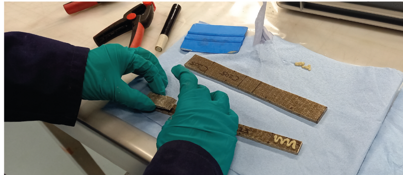
(a) Glueing the composite end tabs on a layup A sample with a two component epoxy adhesive
