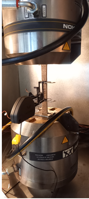
Figure 5.9: Quasi-static tensile test setup in a climate chamber, with a dog bone-shaped sample in the hydraulic wedge clamps, and an extensometer on the sample
