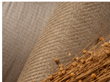
(d) Natural (flax) fibres, on the left a unidirectional sheet and on the right a bidirectional weave (Bcomp, n.d.)
