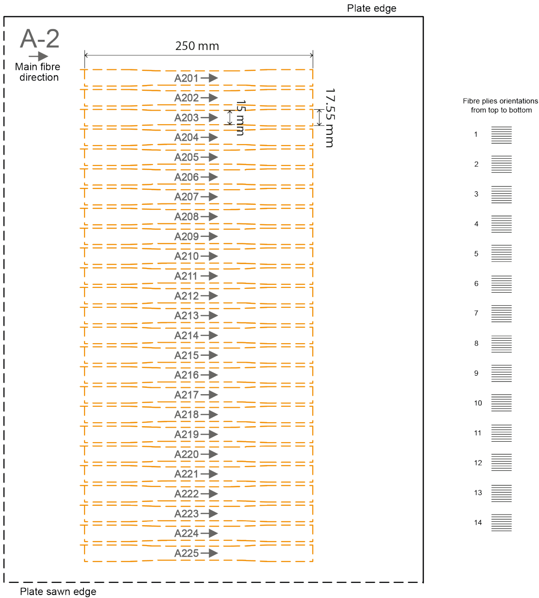
Figure B.4: The samples on plate A-2, the dog bone shaped samples (in orange lines) are cut with a water jet cutter, the black dashed line of the edge plate was the saw line of the original plate
