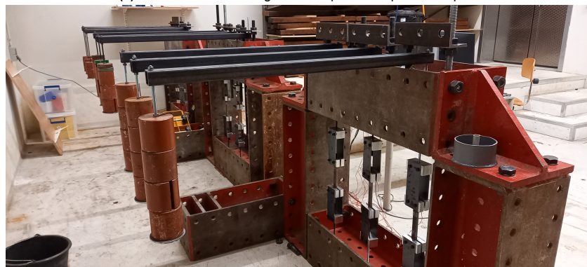
(b) The back view of the long-term creep test setup with samples, with a good view of the lever arm system with the applied weights
