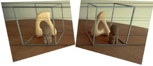
Fig. 11. Rectification of images taken from the same objects but at different locations. Note that after rectification detected features are always horizontally aligned. [40]
