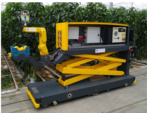
Fig. 3: The SWEEPER sweet pepper harvesting robot by Wageningen University [16], currently the most effective greenhouse harvesting robot.
