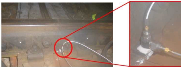
Figure. 4.16: Set-up of accelerometers used to measure impact vibration
