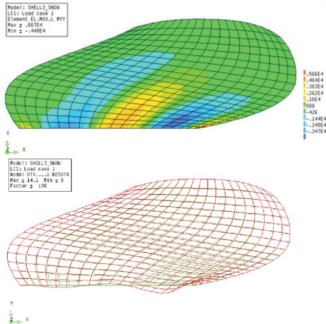
Figure 10.7 The places with the largest deflections are also the places where the largest bending moments are present in the shell.
