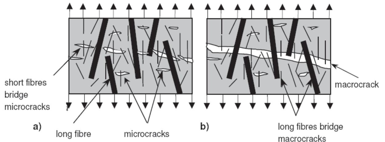
Figure 4.9 The influence of short fibres on bridging micro cracks a) and long fibres on bridging macro cracks b). [13]
