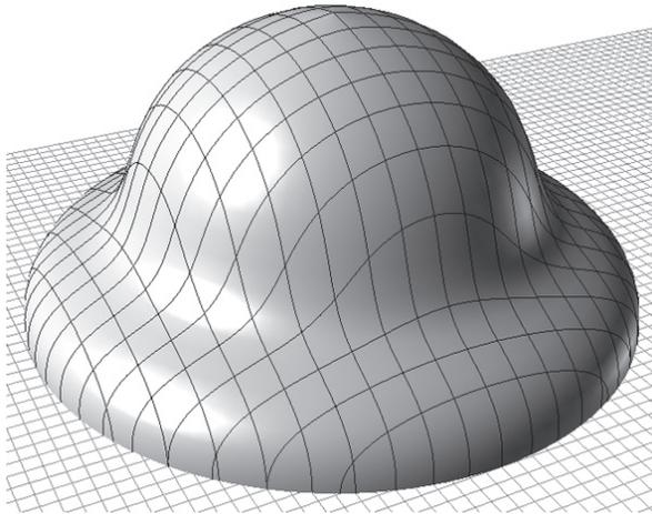
Figure 9.2 Surface of revolution with a projected grid.
