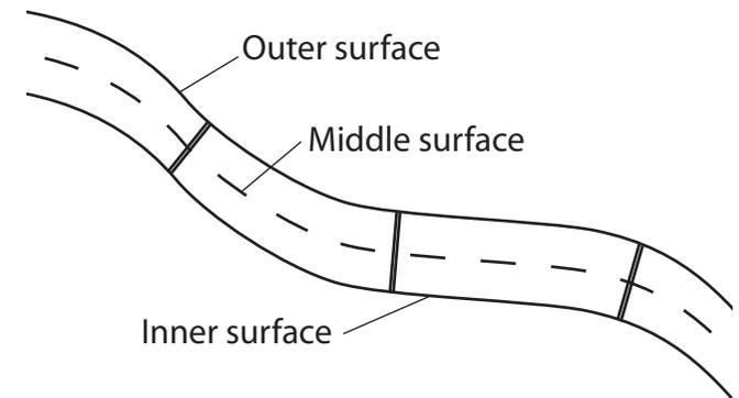
Figure 6.1 A segment of a shell with the three surfaces (inner, outer and middle) that can be distinguished.
