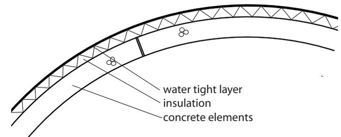
Figure 6.1 Roof package with the insulation on top of the elements.
