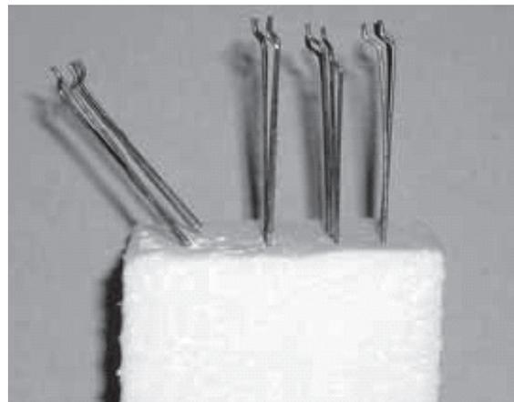
Figure 6.15 Supporting ribbon with fibres. [21]
