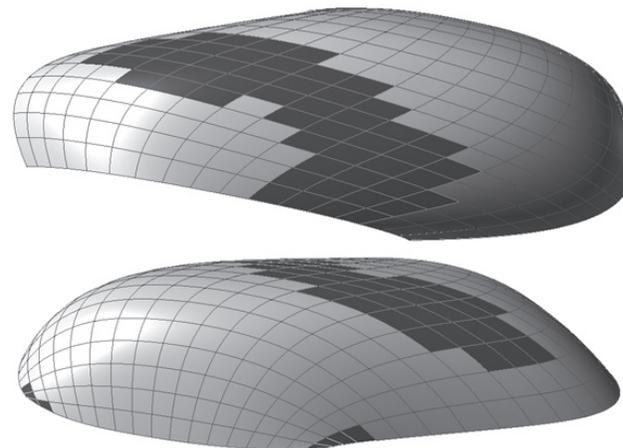
Figure 10.25 The elements of which an angle is determined as too small or too large are marked.
