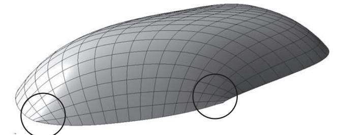
Figure 10.26 The problem areas of the grid the element size and element curvature are marked with the two circles.
