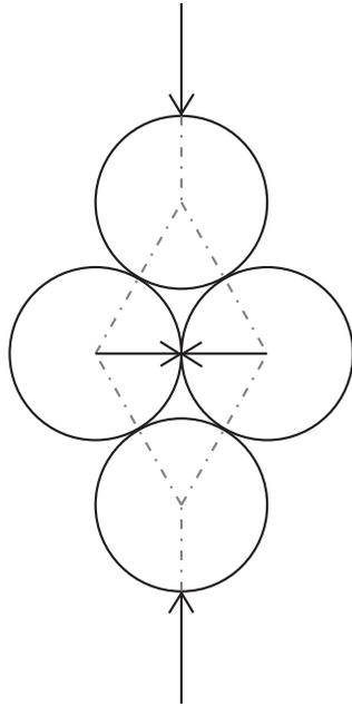
Figure 4.2 Simplified scheme of the force flow in concrete. A large compression force results in a much smaller tension force on the contact surfaces between the grains.
