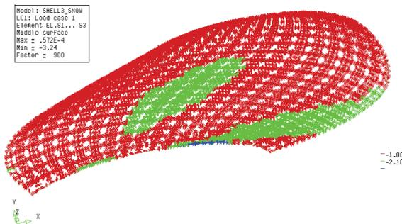
Figure 10.14 Principal stresses in the direction  $\sigma_3$  displayed with the vector representation for load case 2.
