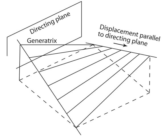
Figure 2.3 Example of a ruled surface.
