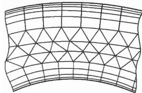
Figure 3.15 A fragment of a hybrid grid. [12]
