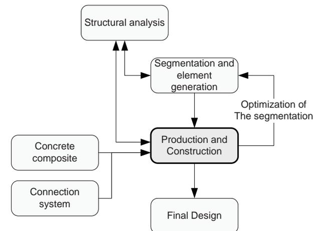
Figure 8.8 The relations of the production and construction process with the other aspects of the design process.
