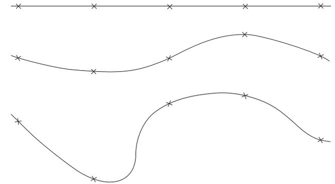
Figure 9.1 A rapid variation in the height of the surface results in a variation in the element size.
