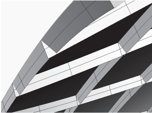
Figure 6.8 Incorrect alignment of the edges with semi-perpendicular edge generation.
