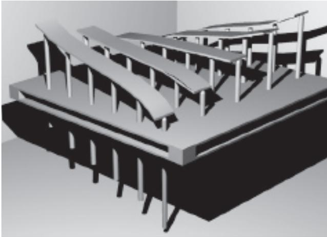
Figure 5.2 Strip mould as designed by H. Jansen with 1 layer of strips. [10]
