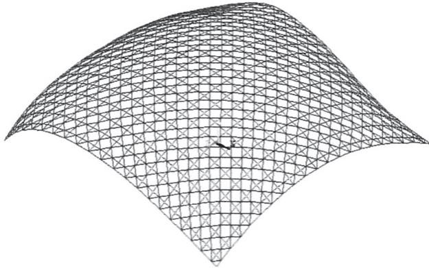
Figure 2.15 Buckling behaviour of a shell with bending stiff connections. [30]
