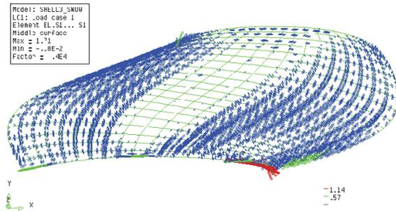
Figure 10.12 Principal stresses in the direction  $\sigma_1$  displayed with the vector representation for load case 2.
