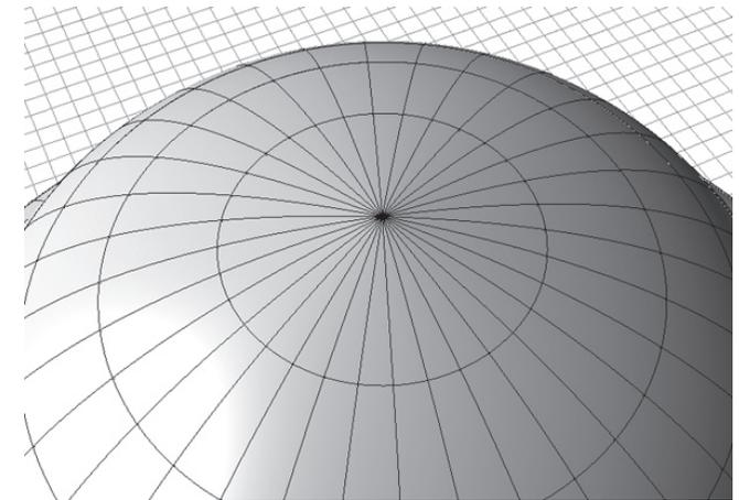
Figure 3.13 The elements in the top of the surface of revolution are generated as triangular elements, with very small angles in top of the surface.
