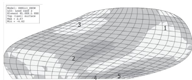
Figure 10.19 The places where the average stresses in the shell are determined are marked with a number.
