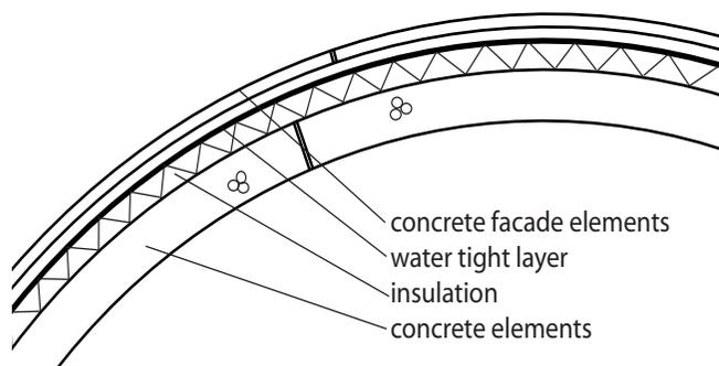
Figure 6.3 Package composition with concrete elements on the inside and outside.
