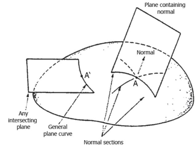
Figure 2.1 Intersection of different planes with a surface. [3]
