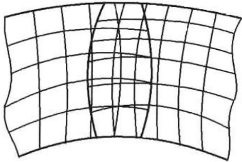
Figure 3.14 Example of an overset grid. [12]
