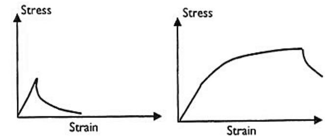
Figure 4.7 Schematic description of strain softening (left) and strain hardening (right) in tension. [1]
