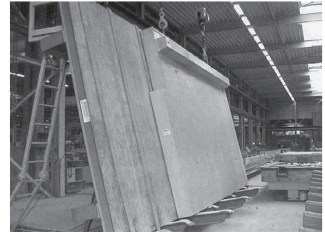
Figure 7.6 Precast concrete element on a turning table. [2]
