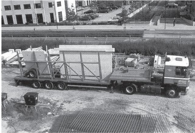
Figure 7.9 Concrete elements on a low loader. [2]
