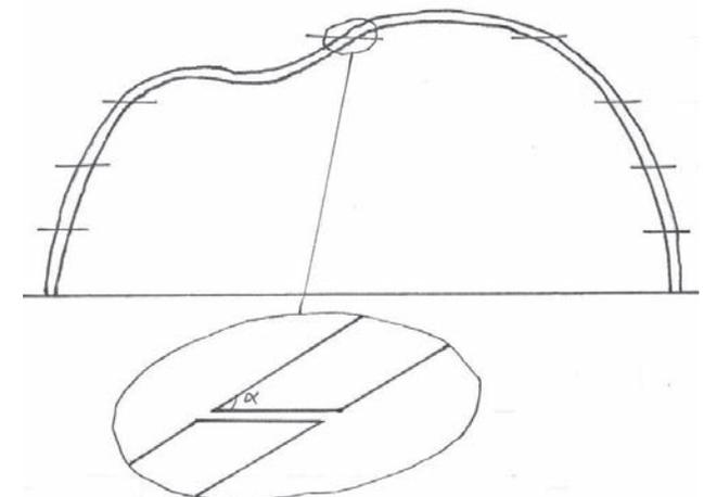
Figure 6.4 Cross-section of an example of a shells that is sliced horizontal in different elements.
