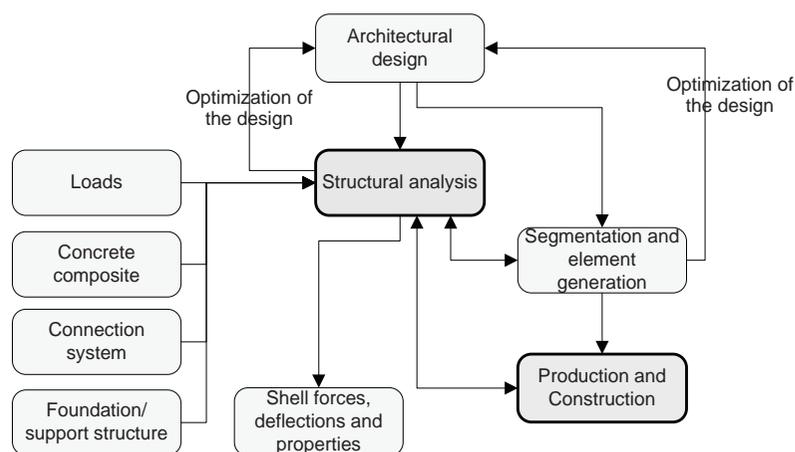
Figure 8.5 Relations of the structural analysis with the other aspects of the design-process.
