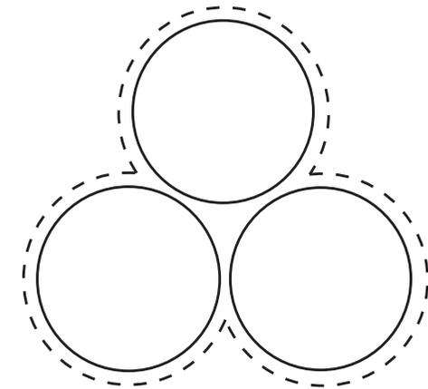
Figure 4.4 'Floating grains' in self compacting concrete. [41]
