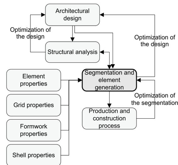
Figure 8.7 Relations of the segmentation and element generation process with the other aspects of the design-process.
