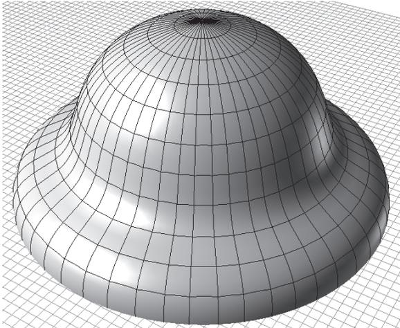
Figure 3.4 Surface of revolution with a Rhino mesh.
