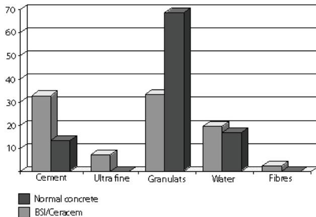
Figure 4.15 Composition of BSI/Ceracem compared to the composition of ordinary concrete. [51]
