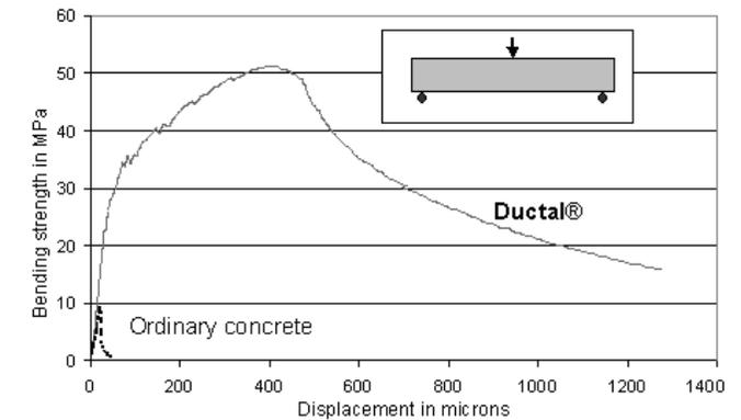
Figure 4.16 The bending strength deflection graph of Ductal compared to normal strength concrete. [52]
