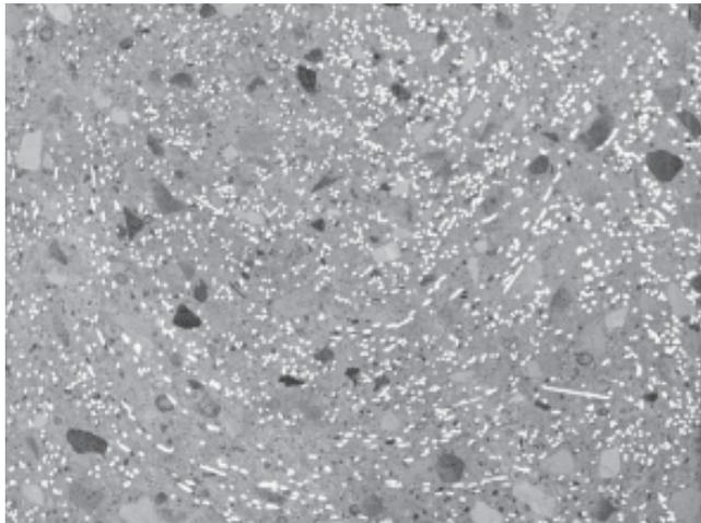
Figure 4.14 BSI/CERACEM in the hardened state, beam cross section of 125 x 125 mm. [11]
