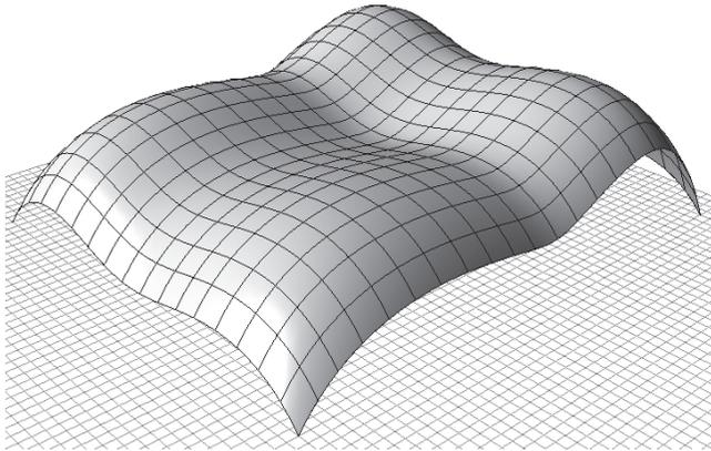
Figure 9.8 A translational grid generated over a surface.
