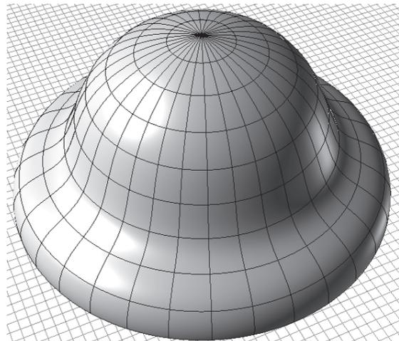
Figure 3.10 Surface of revolution with an isocurve grid. Maximum deviation with rebuilding is 0,00894 m
