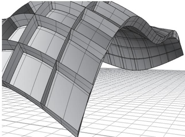
Figure 3.15 This detail of surface 1 shows that the edges of the elements are in torsion.
