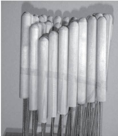
Figure 5.5 Model of the pin bed mould made by M. van Roosbroeck. [19]
