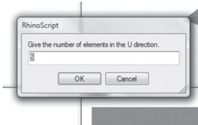
Figure 9.17 The option box in which the user has to give the initial number of elements for the generated grid.
