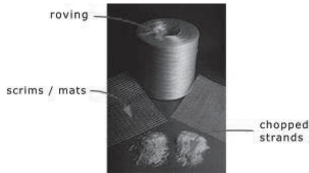
Figure 4.12 Different types of glass fibres. [56]
