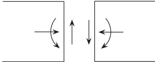
Figure 6.11 The forces that act on the connection between the different elements.
