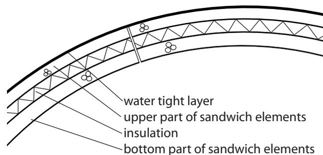
Figure 6.4 Package composition of the shell composed of sandwich elements.
