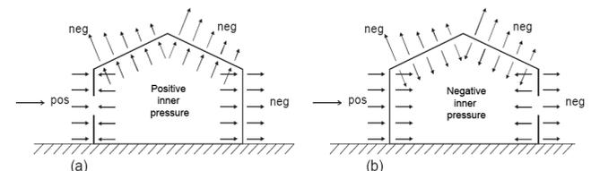
Figure 10.6 Coefficients of the inner pressure on the surface. [15]
