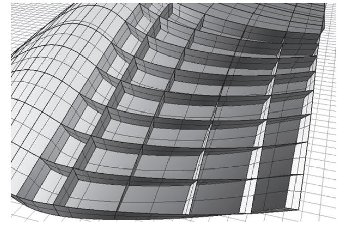
Figure 3.17 This detail of surface 2 shows that these edges are also in torsion.
