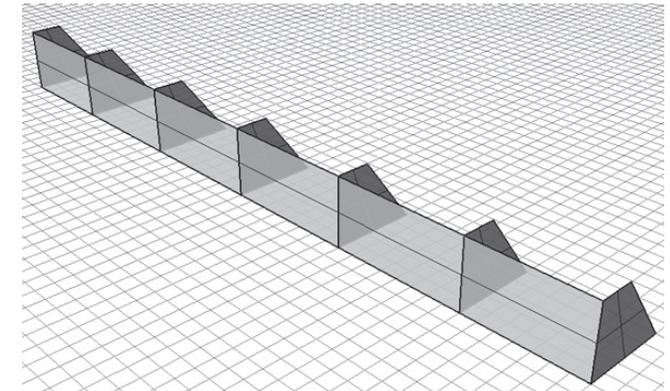
Figure 7.2 Design of the inserts that form the edges of the elements.
