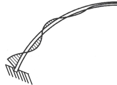
Figure 2.12 Fixed edge conditions induce bending in the shell surface. The bending moments damp out rapidly. [22]
