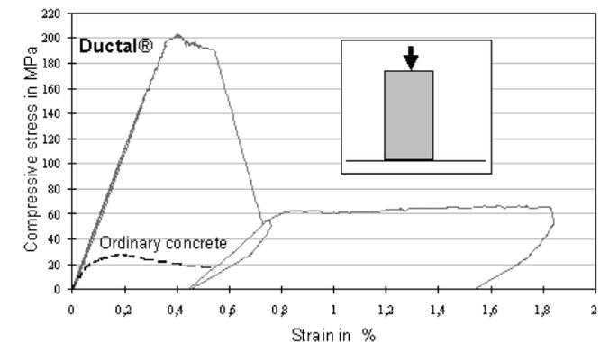
Figure 4.17 The compressive strength strain graph of Ductal compared to normal strength concrete. [52]
