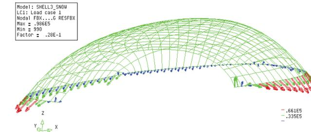
Figure 10.15 Resultants of the reaction forces of the shell for load case 2.
