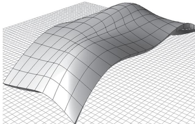
Figure 3.11 Surface 1 with an isocurve grid. Maximum deviation with rebuilding is 0,00693 m
