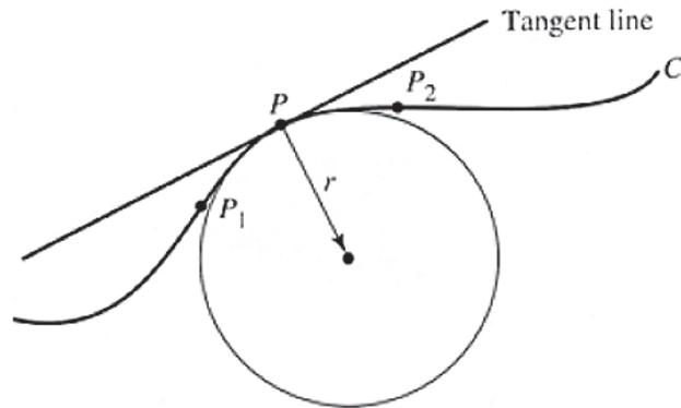
Figure 2.2 Radius of curvature  $r$  of a general curve C. [59]
