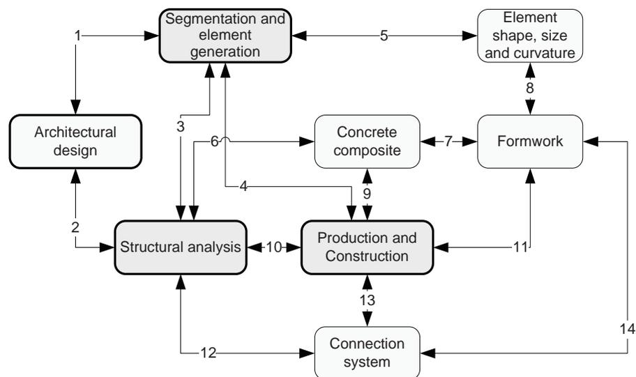
Figure 8.2 The relationship scheme of the relations between the different aspects of the design process.
