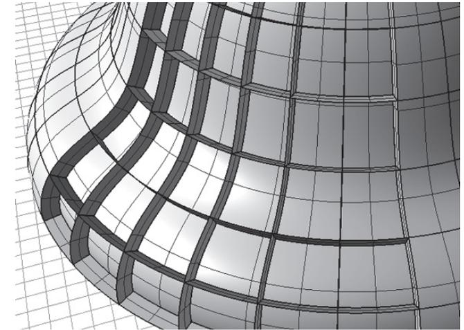
Figure 9.21 Detail of the generated elements of the surface of revolution.
