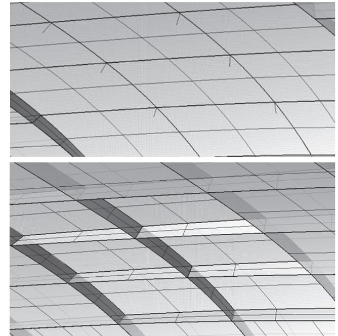
Figure 9.9 Edge generation by first generation the edge lines (above) and the creating the edges (below).
