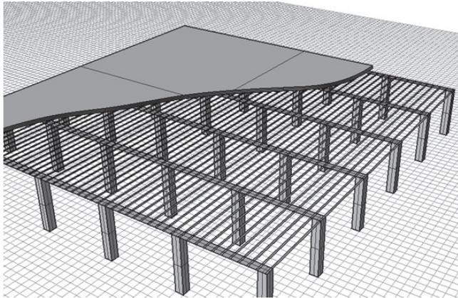
Figure 5.8 A small model that show the idea of the second adjustable mould. In one direction strips are placed on top of the pins. In the other direction a dense net of strips is placed that might be integrated with the rubber cover.
