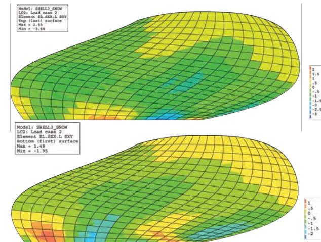
Figure 10.11 The stresses  $\sigma_{xy}$  in the top (above) and bottom (below) of the shell surface due to load case 2 dead load and snow load.
