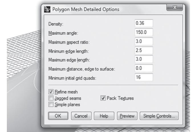
Figure 4.1 The option control box of the Rhino mesh tool.
