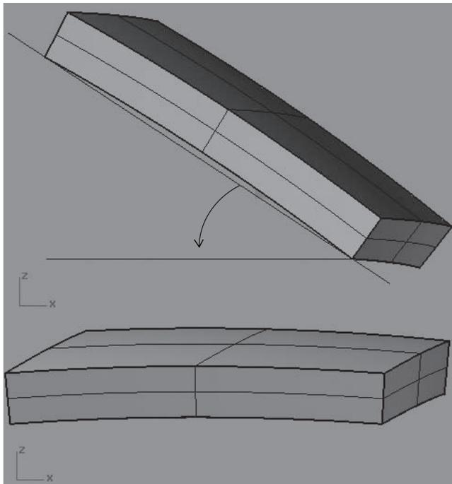
Figure 7.1 The rotation of an element around one axis to the right orientation for the placement on the adjustable formwork. After this rotation the elements has to be rotated around the other axis.
