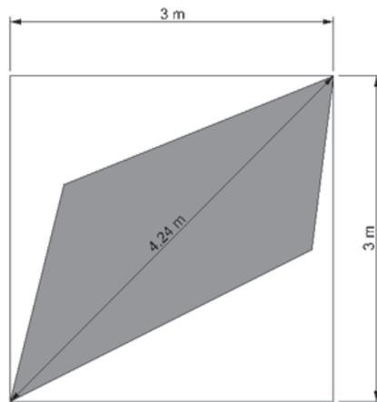
Figure 9.14 The maximum length of the diagonals of the projected element is  $3\sqrt{2} = 4,24 \text{ m}$
