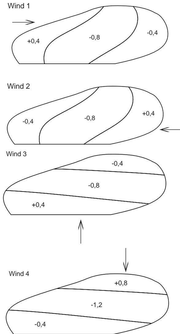
Figure 10.5 Compression coefficients on the surface for the different wind directions.
