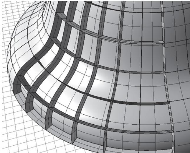
Figure 3.14 The edges of the surface of revolution are almost not in torsion probably due to the regular change of the curvature of the surface.
