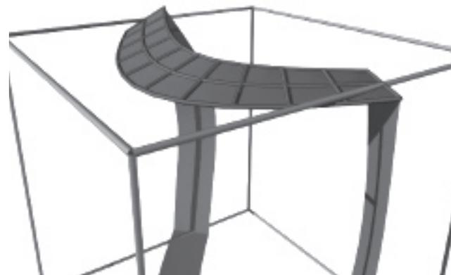
Figure 6.7 A disadvantage of slicing a shell in perpendicular is that the edges are under torsion. [5]
