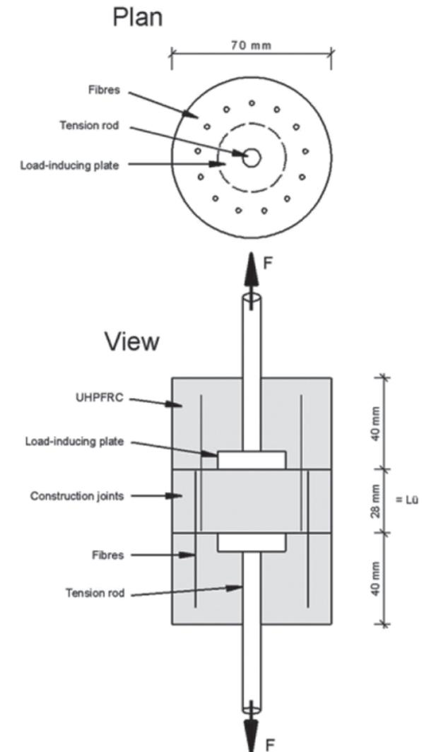
Figure 6.16 Test setup for the test with the fibre reinforced construction joint. [21]
