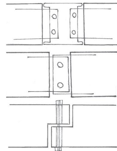
Figure 10.21 Three simple design ideas for a bolted connection.
