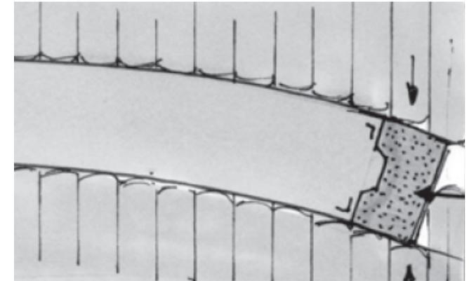
Figure 6.10 The formation of an edge with the insertion of a strip in the pin-bed mould. [19]
