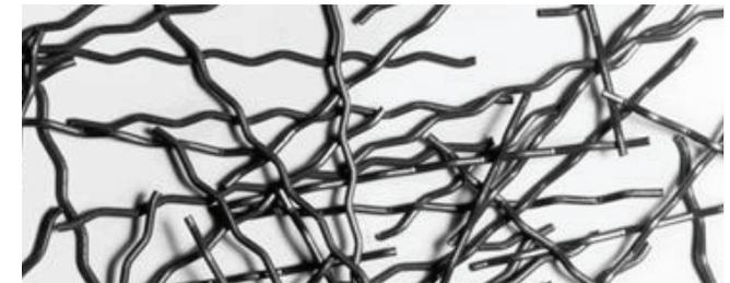
Figure 4.10 Steel fibres.
