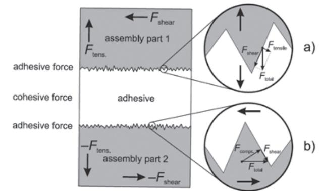
Figure 6.12 Epoxy joint of a rough surface in detail; a) tensile load b) shear stress. [6]
