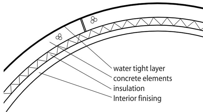
Figure 6.2 Package composition with the insulation under the elements.
