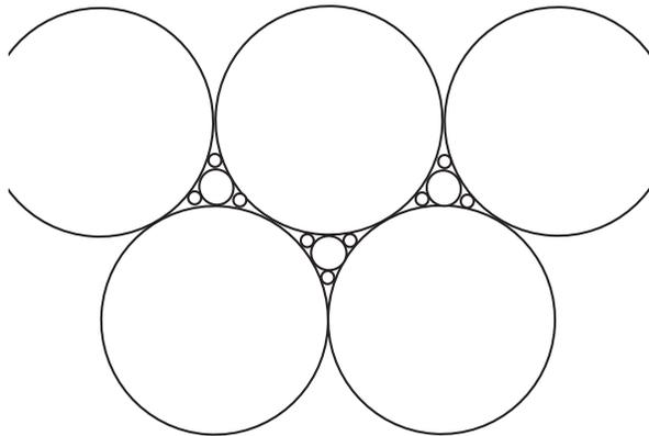
Figure 4.5 Optimal packing arrangement where each grain fills the voids between the larger grains.
