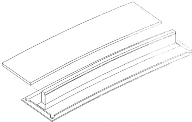
Figure 1.8 Curved T-shape precast concrete element with cover slab (not on scale) [28]
