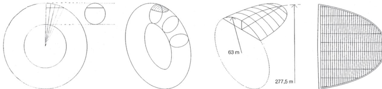
Figure 1.11 Geometry of the roof shell. [28]
