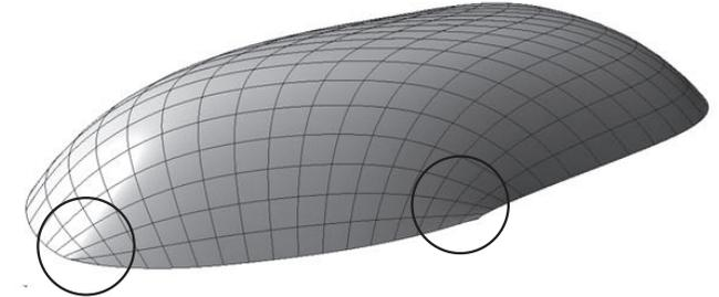
Figure 5.1 The problem areas of the grid the element size and element curvature are marked with the two circles.
