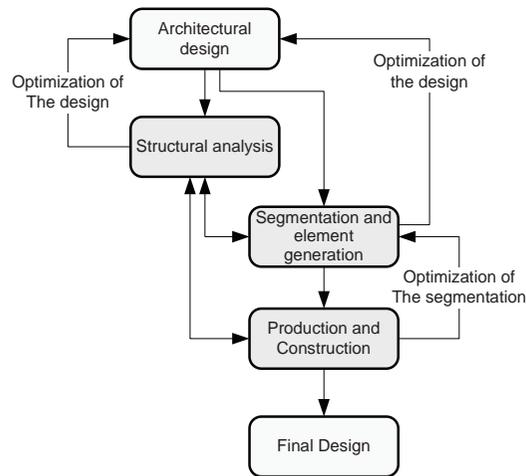
A simplified scheme of the design process for the design of a prefabricated concrete shell structure.
