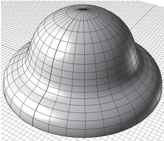
Figure 3.7 Surface of revolution with an isocurve grid.
