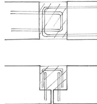
Figure 10.20 Two different options for the design of the wet connection.
