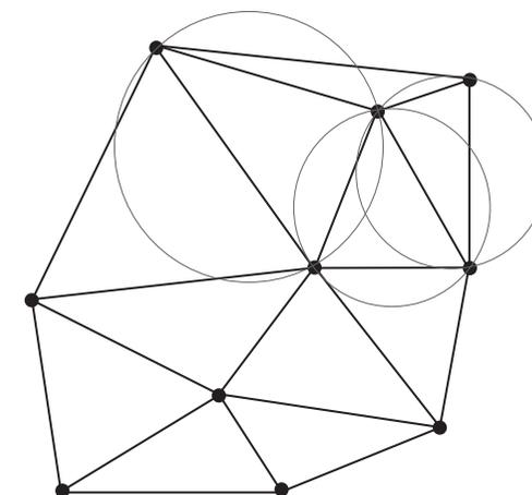
Figure 3.8 Delaunay triangulation with empty circumcircles.
