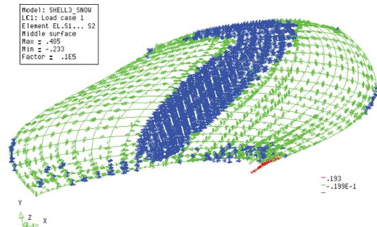
Figure 10.13 Principal stresses in the direction  $\sigma_2$  displayed with the vector representation for load case 2.
