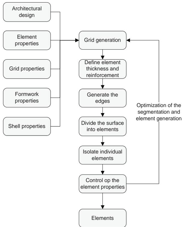
Figure 8.6 The different actions in the segmentation and element generation process.
