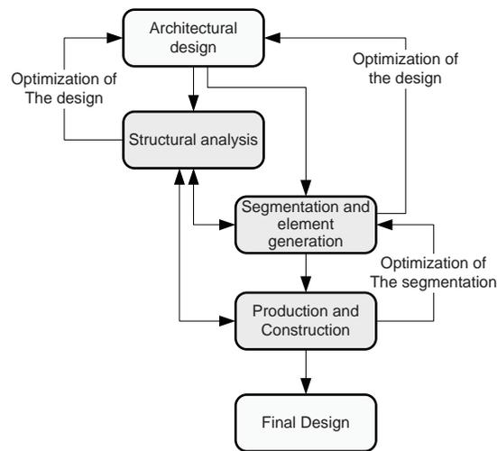
Figure 8.3 The simplified design process of a prefabricated concrete shell structure.
