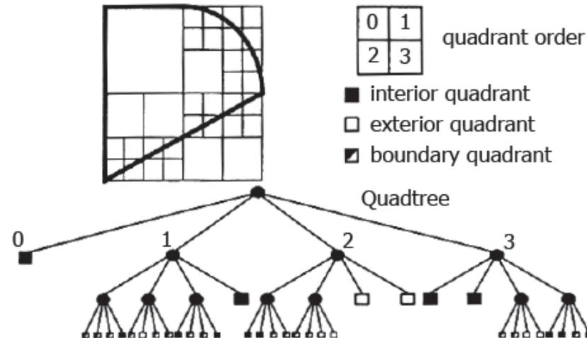
Figure 3.7 Example of the octree approach. [23]
