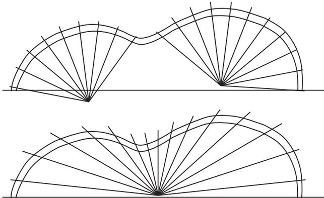
Figure 6.9 Two cross-sections of a shell that is cut radial in different elements.
