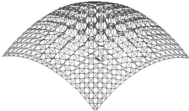
Figure 2.16 Buckling behaviour of a shell with hinged connections. [30]
