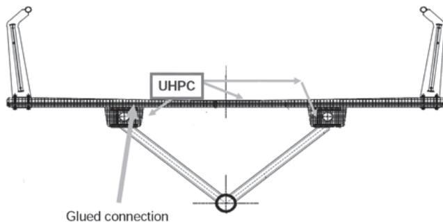
Figure 6.14 Cross-section of the Gartnerplatz bridge in Kassel. [6]
