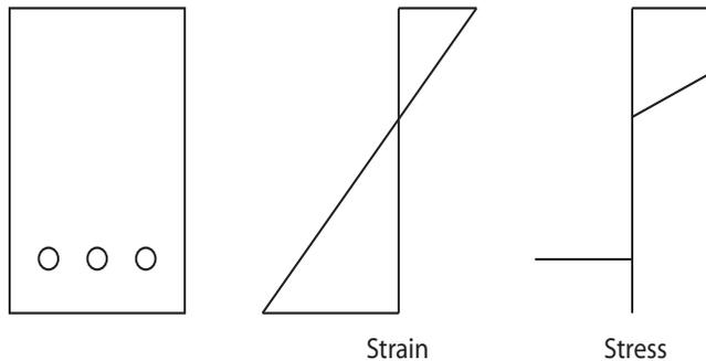
Figure 4.3 The strain and stress distribution of a reinforced concrete beam in bending show that the tension in the lower part of the beam is taken by the reinforcement and compression in the top is taken by concrete.
