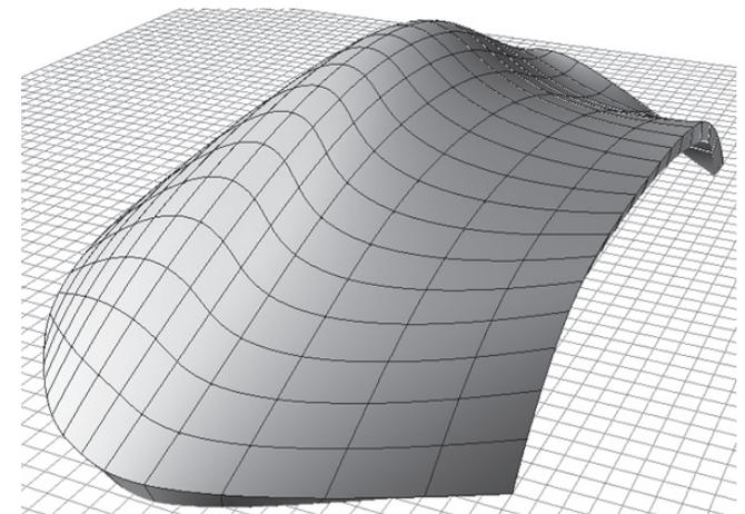
Figure 3.12 Surface 2 with an isocurve grid. Maximum deviation with rebuilding is 0,00589 m
