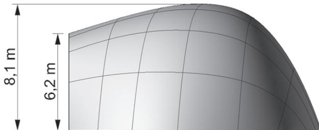
Figure 10.2 Side view of the shell design with some dimensions.
