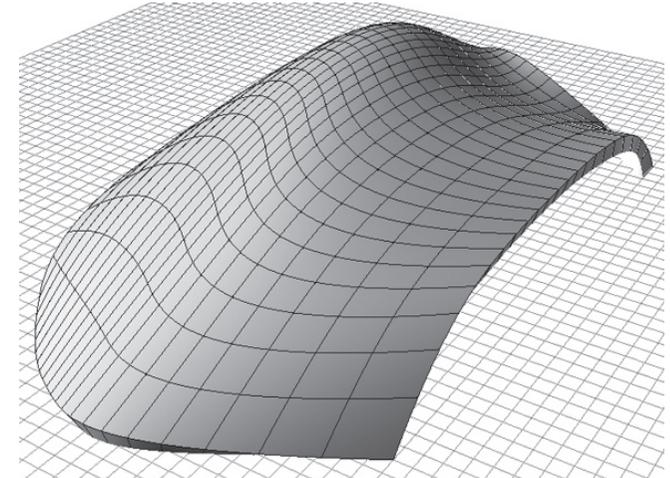
Figure 3.9 Surface 2 with an isocurve grid.
