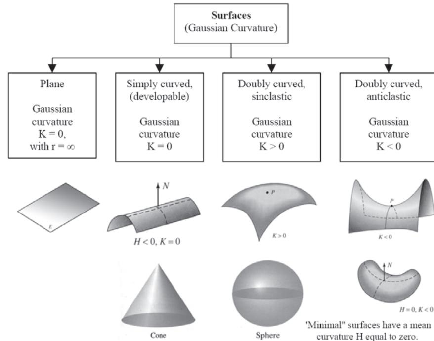
Figure 2.5 Surface classification by Gaussian curvature. [59]
