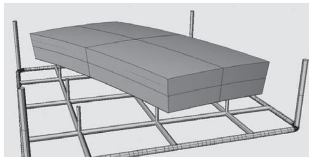
Figure 7.7 Model of the frame to store the double curved elements.
