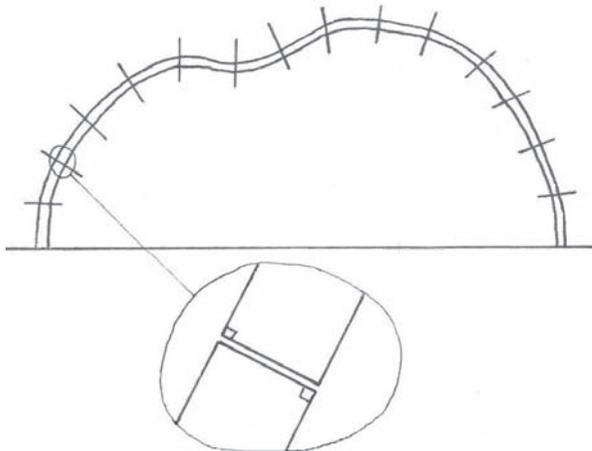
Figure 6.6 Cross-section of an example of a shell that is sliced perpendicular to the surface.
