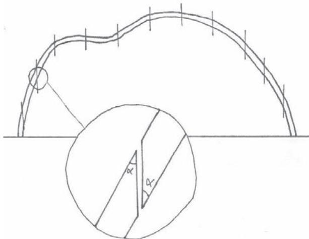
Figure 6.3 Cross-section of an example of a shells that is sliced vertical in different elements.
