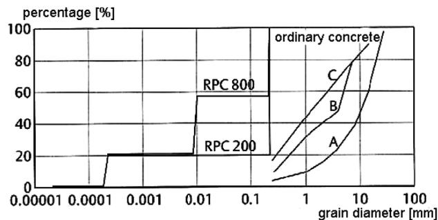
Figure 4.6 The discontinuous distribution of grain sizes of high performance concrete compared to the continuous distribution of grain sizes of ordinary concrete. [4]
