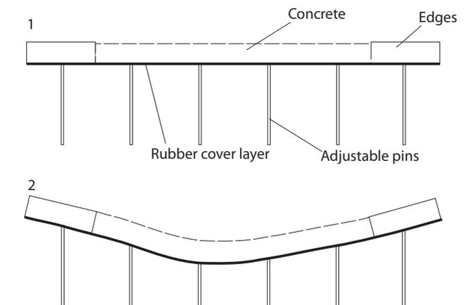
Figure 7.3 Casting principle of the adjustable mould.
