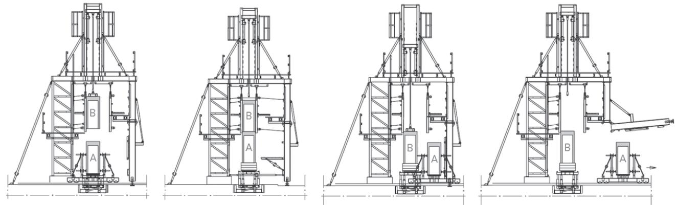
Figure 1.25 Schematic representation of the construction process of the element for the tollgate canopy. [61]
