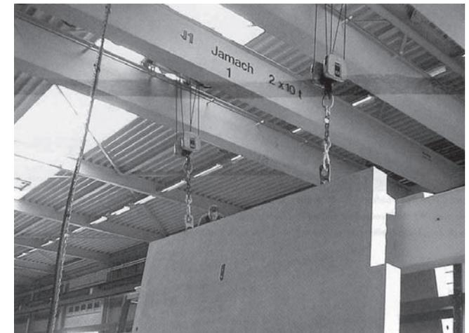
Figure 7.8 Element transported with a crane in the factory. [2]
