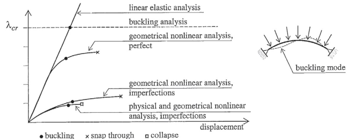
Figure 2.14 Shell finite elements analysis of a shallow dome. [24]
