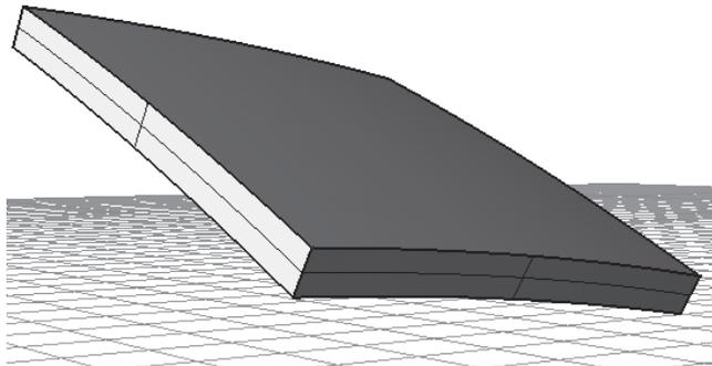
Figure 9.10 Element with edges generated according to the perpendicular edge generation method.
