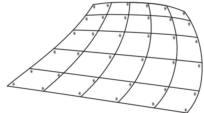
Figure 9.16 In a grid only the angle marked with a  $*$  have to be measured to know the size of all angles between the edges of the elements.
