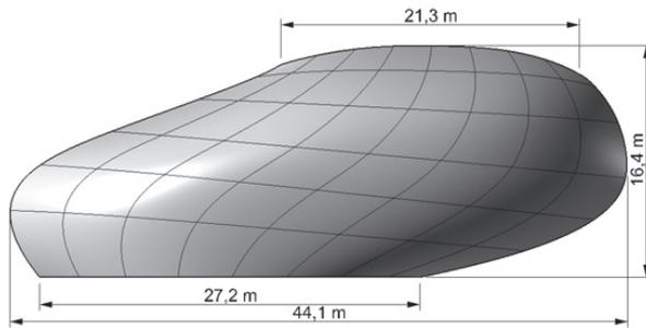
Figure 10.1 Top view of the shell design with some dimensions.
