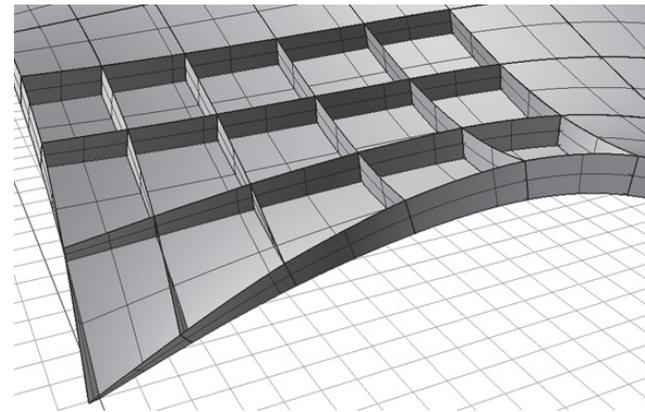
Figure 3.16 This detail of surface 1 shows that the torsion of the edge is larger when the curvature of the surface is larger.
