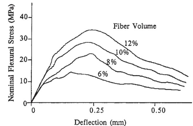
Figure 4.13 Typical flexural stress-deflection behaviour of SIFCON. [27]
