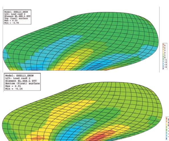
Figure 10.10 The stresses  $\sigma_{yy}$  in the top (above) and bottom (below) of the shell surface due to load case 2 dead load and snow load.
