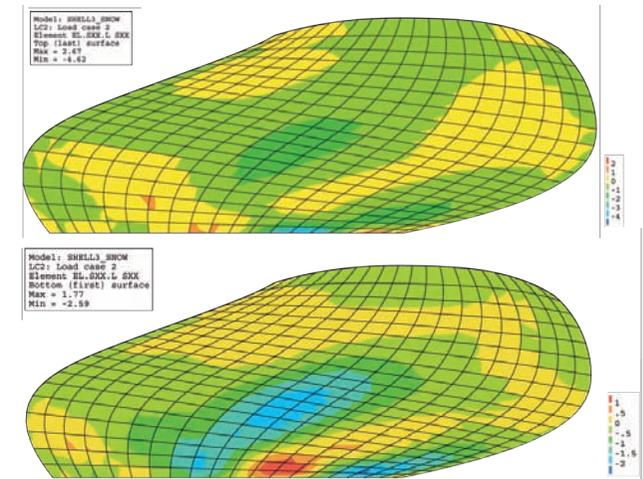
Figure 10.9 The stresses  $\sigma_{xx}$  in the top (above) and bottom (below) of the shell surface due to load case 2 dead load and snow load.
