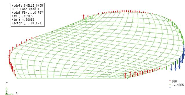
Figure 10.22 Horizontal support reactions in the y direction for load case 2.
