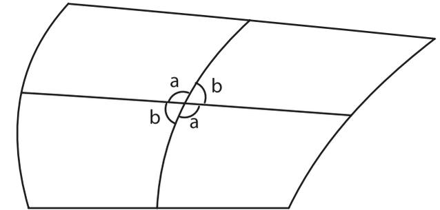
Figure 9.15 This section from a grid show that the angles  $a$  and the angles  $b$  are equally sized. Besides this the size of angle  $a + b$  is always equal to 180 degrees.
