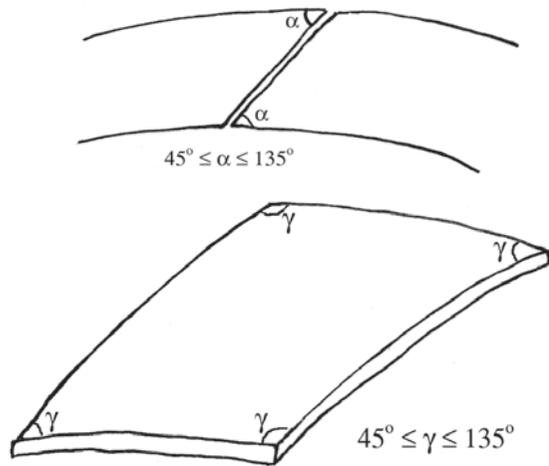
Figure 6.2 Minimum and maximum angle in the cross-section (above) and in the plane of the element (below).
