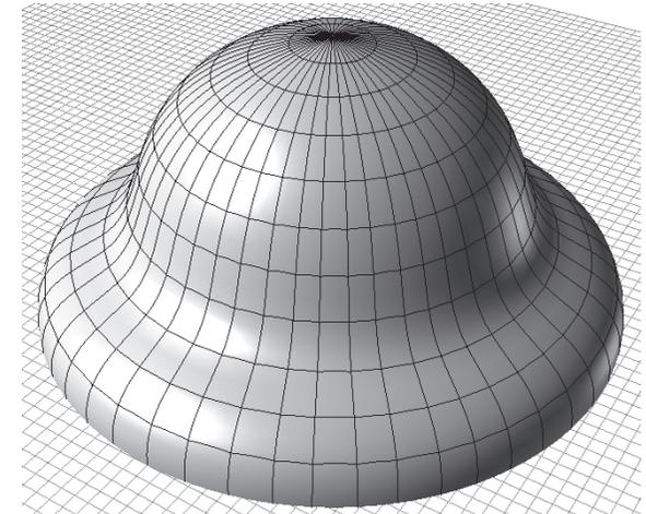
Figure 9.6 Surface of revolution meshed with the Rhino meshing tool.
