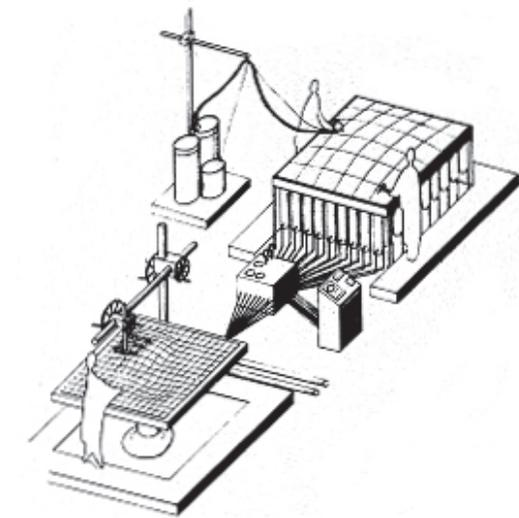
Figure 5.1 Renzo Piano's idea for an adjustable formwork for the fabrication of double curved elements. [5]
