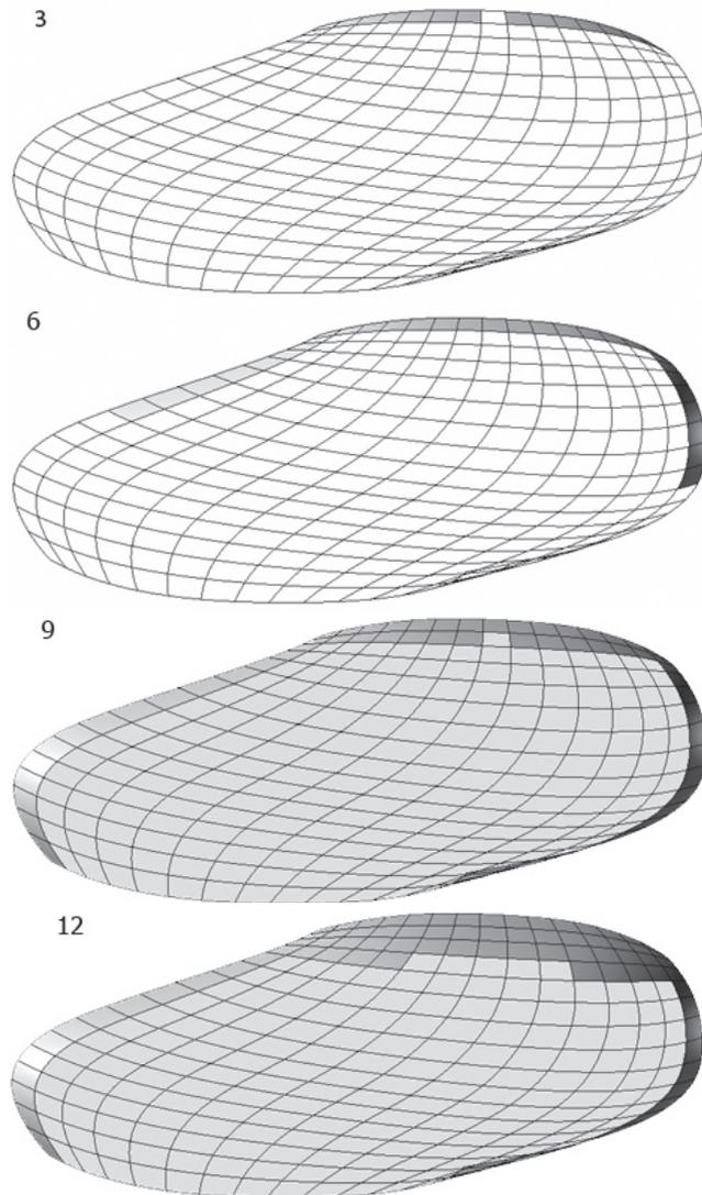
Figure 10.29 Building sequence of the shell.
