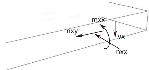
Figure 10.18 The different types of forces that are present in the connection.
