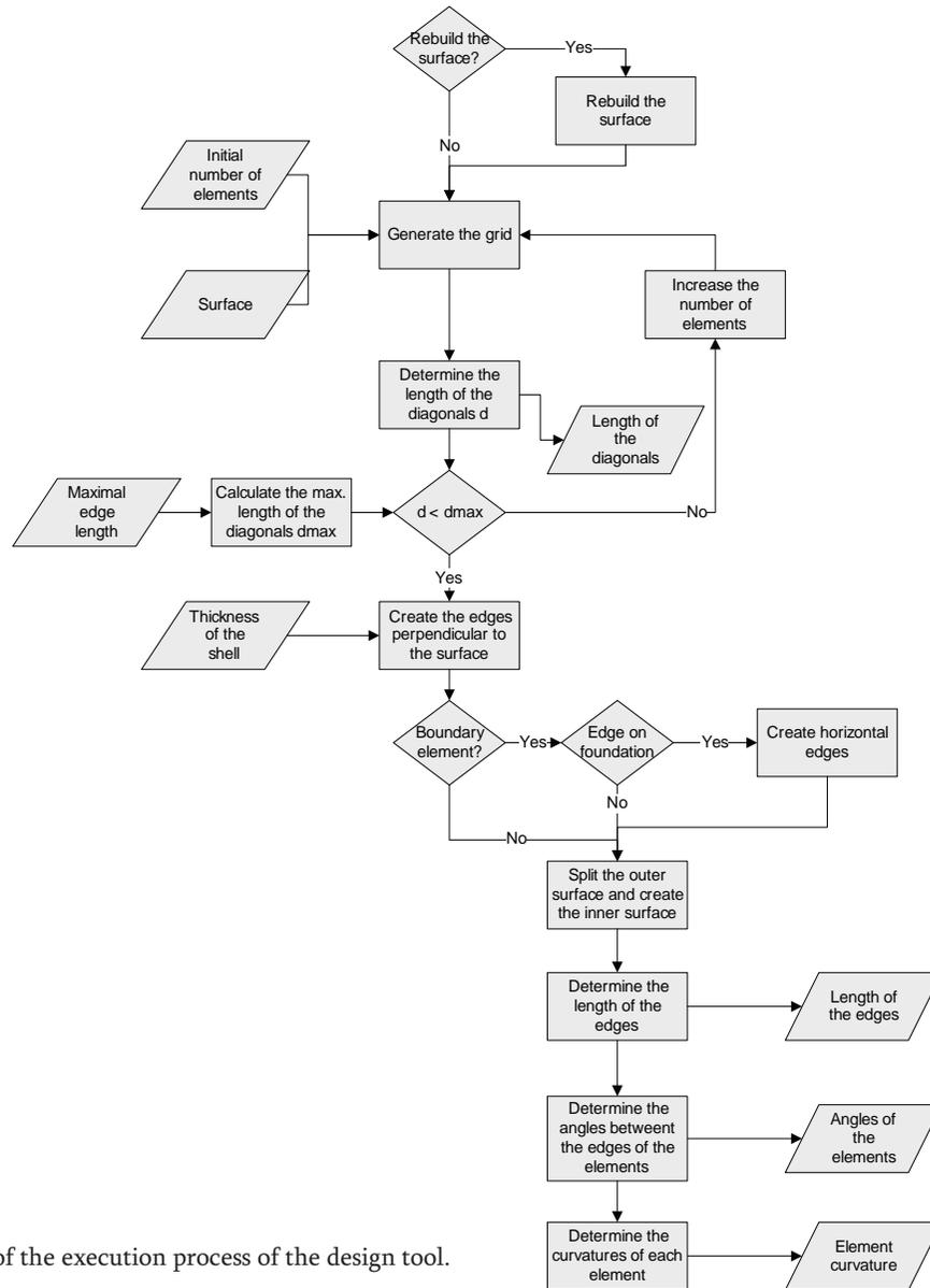
Figure 9.18 Diagram of the execution process of the design tool.
