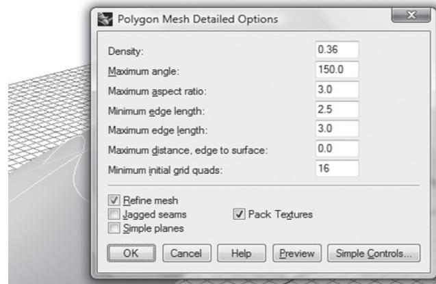
Figure 9.4 The option control box that is used to control the settings for the mesh generation in Rhino.
