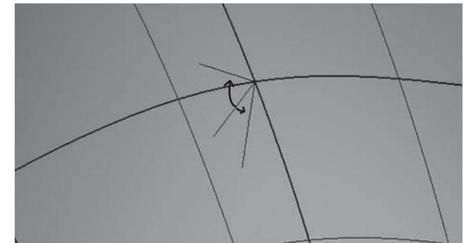
Figure 9.12 The normal vector of the surface will always be rotated in the plane of a grid line to the horizontal or vertical direction. The rotated edge line is still perpendicular to the other grid line.
