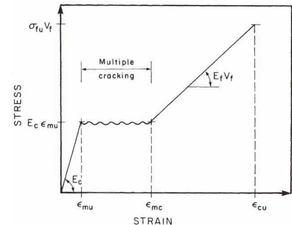
Figure 4.8 Schematic description of the stress-strain curve, based on the ACK-model. [1]
