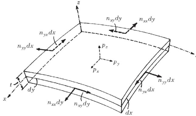
Figure 2.10 Stress resultants and load components on a shell element. [3]
