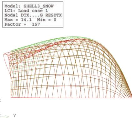
Figure 10.8 Side view of the shell with the resulting deflections of the shell surface due to both the dead load and snow load.
