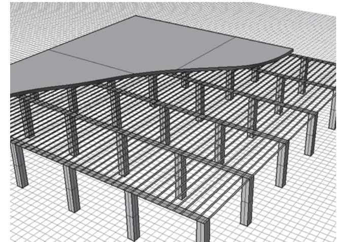
Model of the adjustable formwork as it is in development at the moment.
