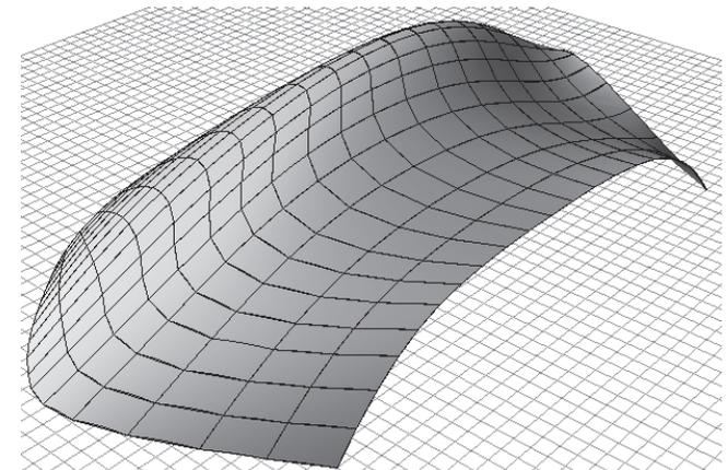
Figure 9.5 Surface 2 meshed with the Rhino meshing tool.
