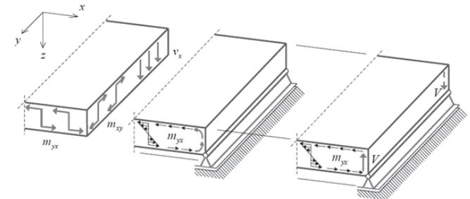
Figure 10.16 The development of local shear forces due to torsional moments  $M_{xy}$  in the shell.
