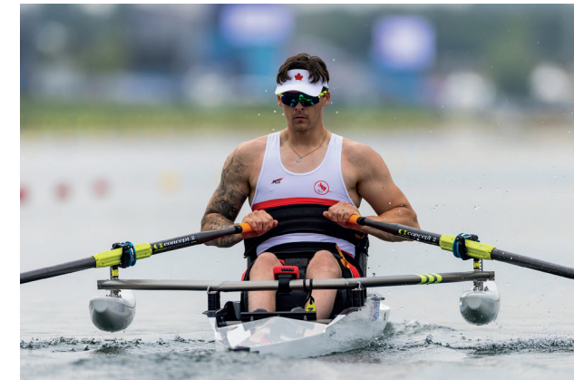
Figure 13. Pontoons attached to a rowing boat (Canadian Paralympic Committee, n.d.)
