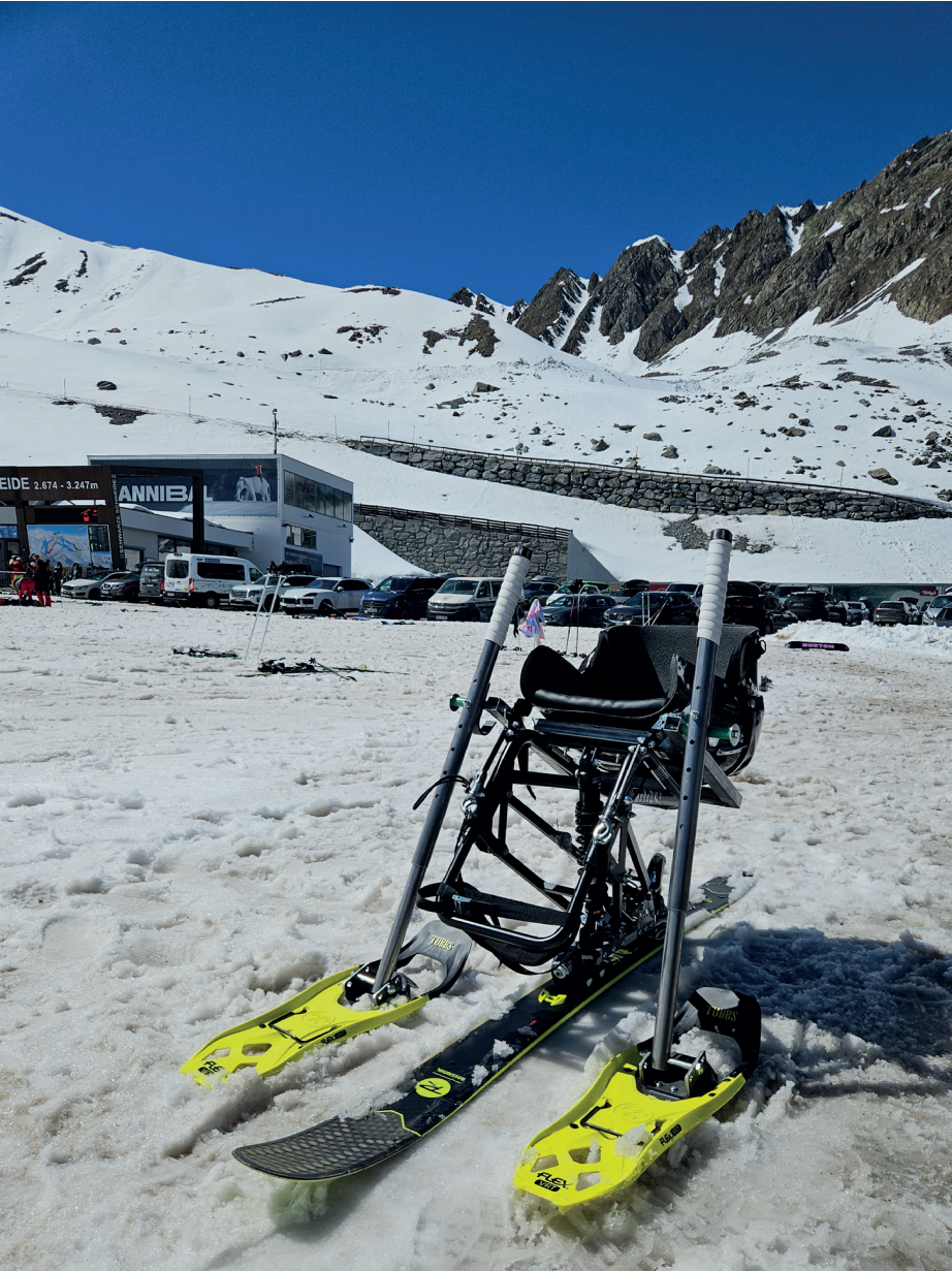
Figure 48. Prototype during on snow usability testing
