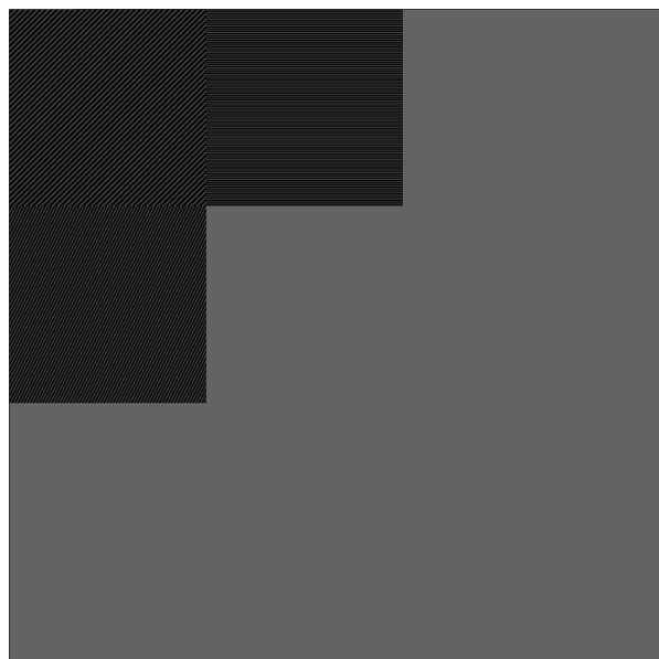
Figure 5.16: Illustration of the steering mechanism and their actuated pixels for the situation illustrated in Figure 5.15. The surfaces allocated to each beam is large enough to not cause noticeable diffraction of the beams. The steering system used has a 10x10 micro mirror resolution and the figure shows the phase field.
