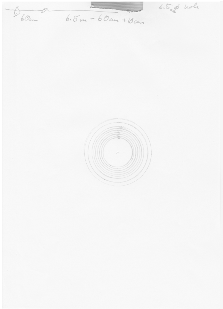
Figure B.18: The trace of dark rings for a 532 nm expanding beam diffraction through a 6.5 mm hole at a distance of 5.74 m. The outer circle was measured with a caliper to be 65.8 mm from the outside line (top down).
