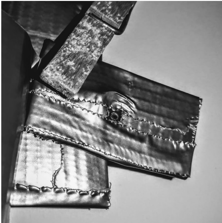
Figure 3.20: Shown is a close-up of one of the diffraction holes, in this case the perf-board. Shown is how the other holes are covered to not interfere with the diffraction pattern.
