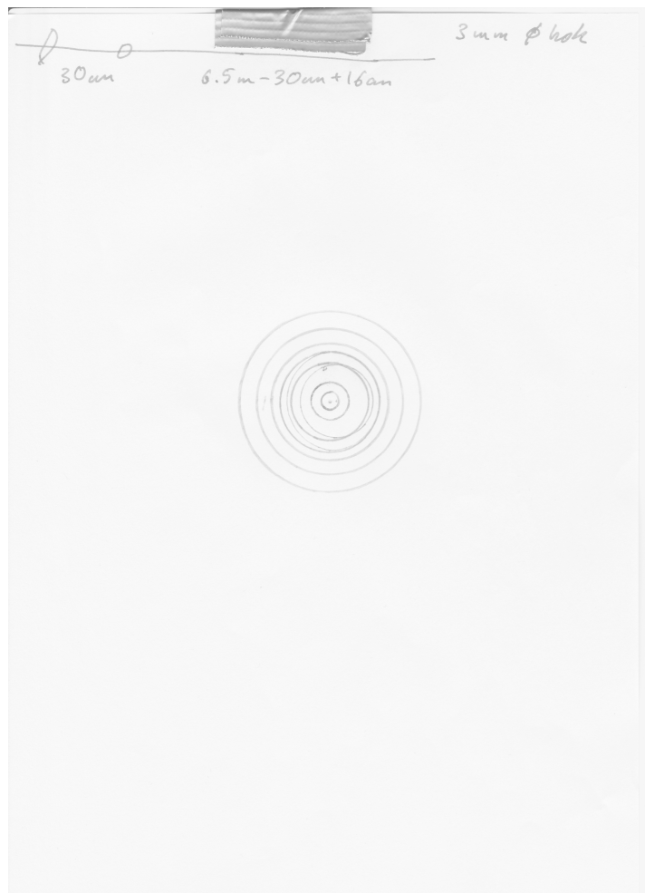
Figure B.12: The trace of dark rings for a 532 nm expanding beam diffraction through a 3 mm hole at a distance of 6.04 m. The inner circle was measured with a caliper to be 61.0 mm from the inside line.
