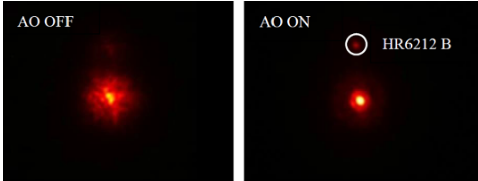
Figure 4.4: This image was taken from ALPAO[2] on their webpage on "Adaptive optics applications" url: https://www.alpao.com/adaptive-optics/alpao-applications.html . It shows an example of a scintillated image of a star left and a corrected image right. As can be seen, the scintillated image contains numerous bright spots and a distribution of the light over a larger area.
