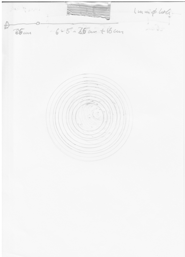
Figure B.6: The trace of dark rings for a 532 nm expanding beam diffraction through a 1 mm hole at a distance of 6.08 m. The inner circle was measured with a caliper to be 15.6 mm from the inside line.
