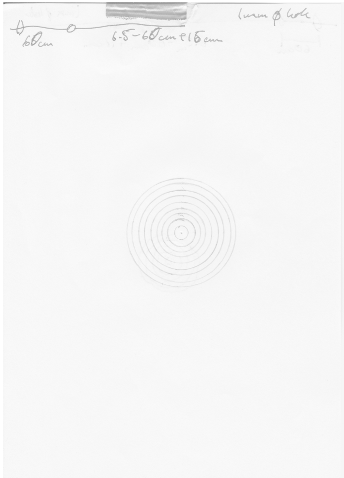
Figure B.9: The trace of dark rings for a 532 nm expanding beam diffraction through a 1 mm hole at a distance of 5.64 m. The outer circle was measured with a caliper to be 68.4 mm from the outside line.
