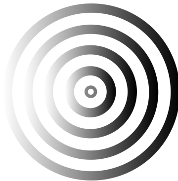
Figure 3.4: Illustration of an oblique spherical wave, with the color depth an illustration of the amplitude of the wavefront. As can be seen, the majority of the wave energy is propagated to the right of the wavefront, while none of the energy is propagated to the left.
