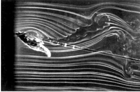
(a) LEV visualisation on a hawkmoth wing; figure adapted from Ellington et al. [37]
