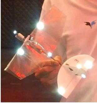
Figure 5.2: Location on the ornithopter of the retro-reflective markers used to track the position.
