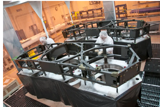
(b) Structural wing sections of the mirror backplane.
