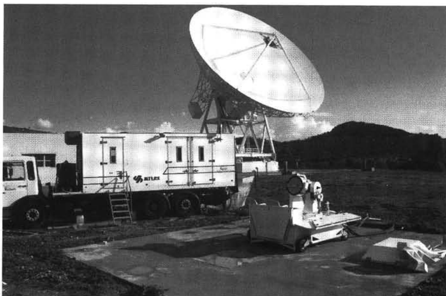
Figure 2.4 The transportable laser ranging system MTLRS-2 observing at Noto, Sicily, near the geodetic VLBI telescope of the Italian Space Agency.
