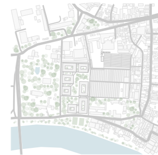
PHASE 2 Demolition of informal settlement, replacement of government ground, new infrastructure and green boulevard, estimated: 144 new dwellings, 70 new shops
