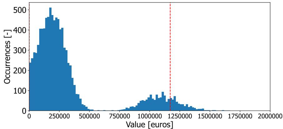
Figure 4.7: Results of a Monte Carlo analysis performed for the functional component of the residual value of the case if the choice is made to directly renovate the roads that have a lifespan shorter than the contract period of 15 years. Represented discounted to 2020 euros.
