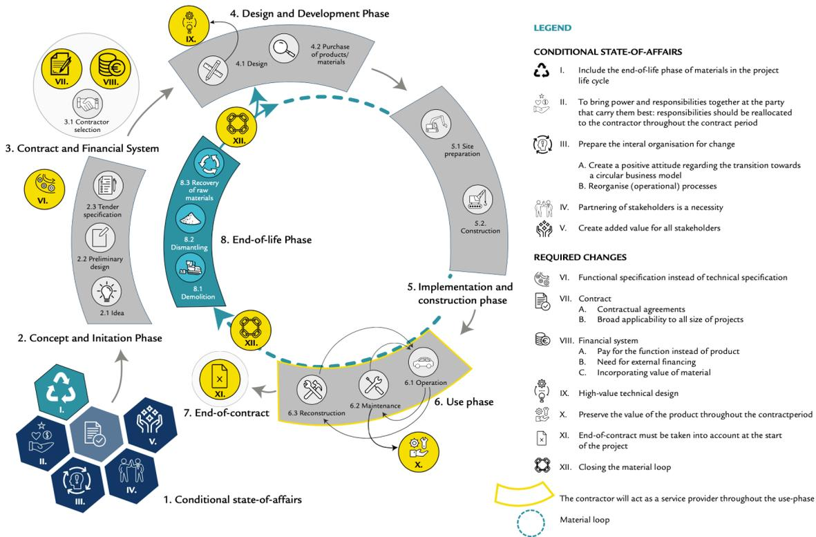
Figure 2.2: Model for incorporating PSS characteristics in infrastructure projects. It shows the adapted project life cycle on the left and reveals where the conditional states of affairs and required changes (stated on the right) should be addressed in yellow. Adopted from (Huizing, 2019).
