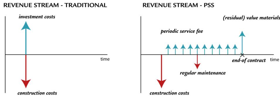
Figure 2.3: Revenue streams for infrastructure projects from a contractor's perspective. The left graph shows the traditional model revenue stream, whereas the right graph shows the revenue stream when a PSS model is applied. Adopted from (Huizing, 2019).
