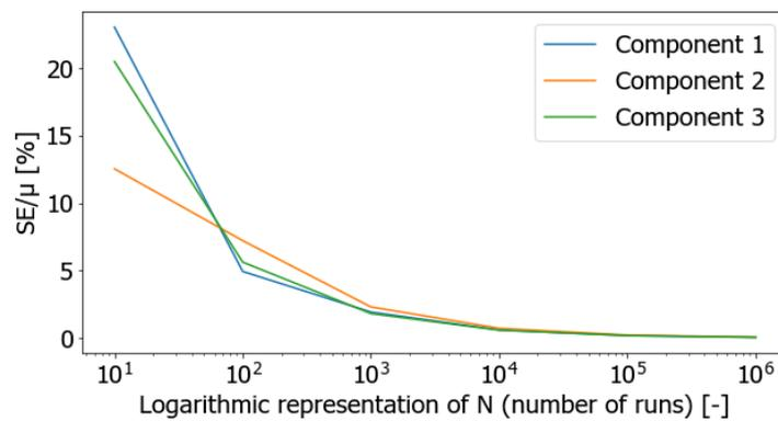
Figure 3.4: Graphical representation of the  $SE/\mu$  of the results of the MCA for each of the three components as set out by the initial design Section 4.2, showing the relative deviation is below 1% for all components for the number of runs of 10.000.
