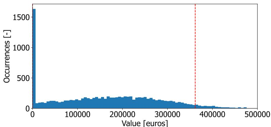
Figure 4.6: Results of a Monte Carlo analysis performed for the functional component of the residual value of the case if the choice is made not to renovate the roads that have a lifespan shorter than the contract period of 15 years. Represented discounted to 2020 euros.
