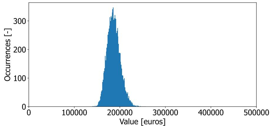
Figure 4.5: Results of a Monte Carlo analysis performed for the physical component of the residual value of the case using CBS data as used for the other components, resulting in a lower spread. Represented discounted to 2020 euros.
