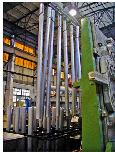
Fig. 1.1. Vertical DC casting process: (a) schematic of a DC caster [8] and (b) an example of DC-cast billets.
