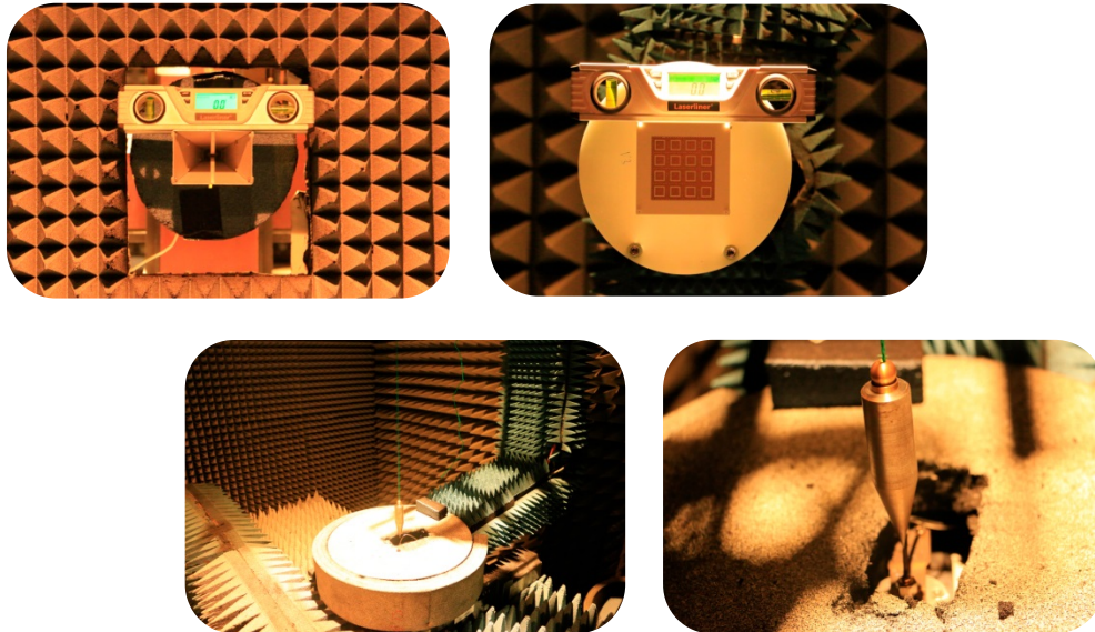
Figure 6-9 – Antenna Positioning using a Spirit Level (Top) and a Plumb Line (Bottom)
