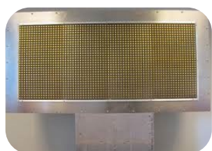
Figure 1-8 – CASA Phase-Tilt Weather Radar [24]
