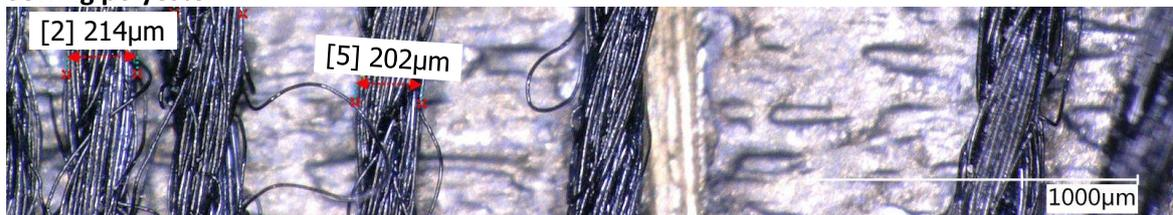
Figure 55 Some examples of the measured thread diameters for crochet polyester, extra strong sewing polyester and sewing polyester.
