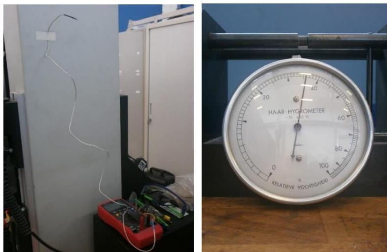
Figure 26 Digital thermometer (left) and analogue hygrometer (right).
