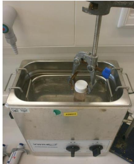
Figure 13 Before the suspension was deposited on the substrates the suspension jar was put in an ultrasonic bath (VWR ultrasonic cleaner) for 2 minutes at room temperature to break agglomerates of spheres.
