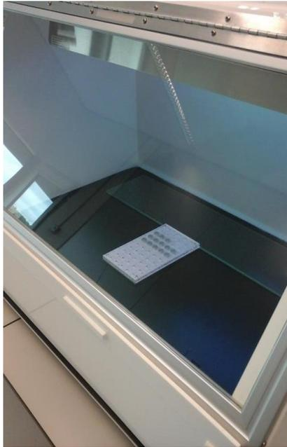
*Figure 6 Fume cabinet with a UV light source.
