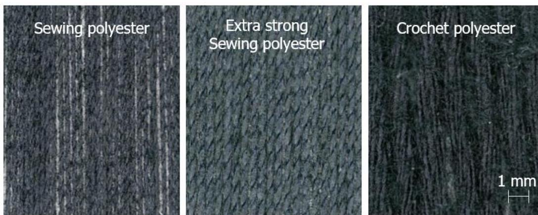
Figure 8 Polyester substrates made of three different threads: sewing polyester, extra strong sewing polyester and crochet polyester. See Table 1 for the thread specifications.
