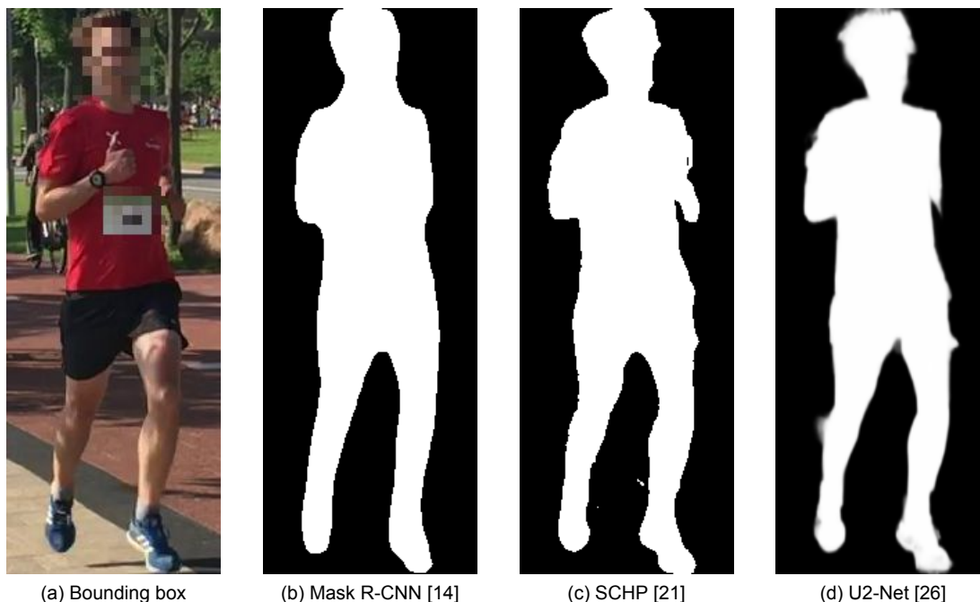
Figure 5.1: Comparison between segmentation methods. (a) bounding box, (b) instance segmentation, (c) human semantic parsing, (d) salient object detection.
