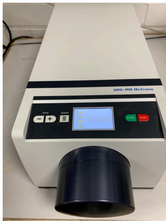
Figure 31: McCrone micronising mill used during this study. Used to reduce the particle size of Kittilä samples and thin disk samples to <5\mu\text{m} in preparation for XRD analysis.
