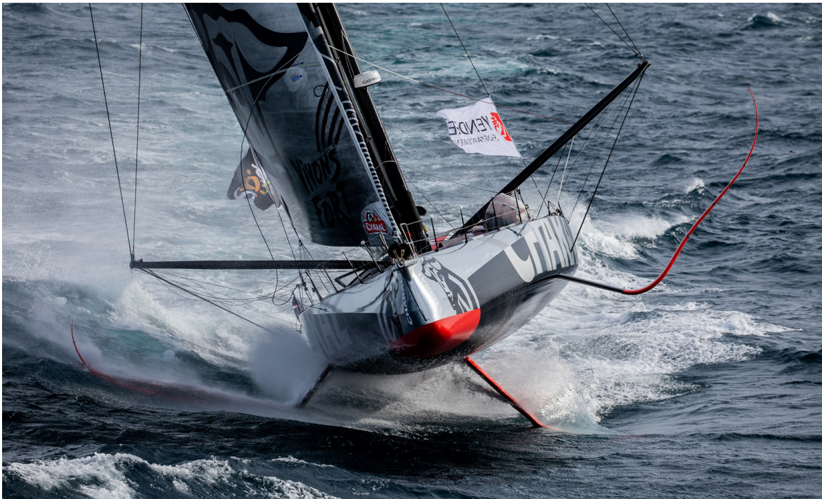
Figure 1.1: IMOCA 60, with surface piercing hydrofoil (Editor, 2020)
