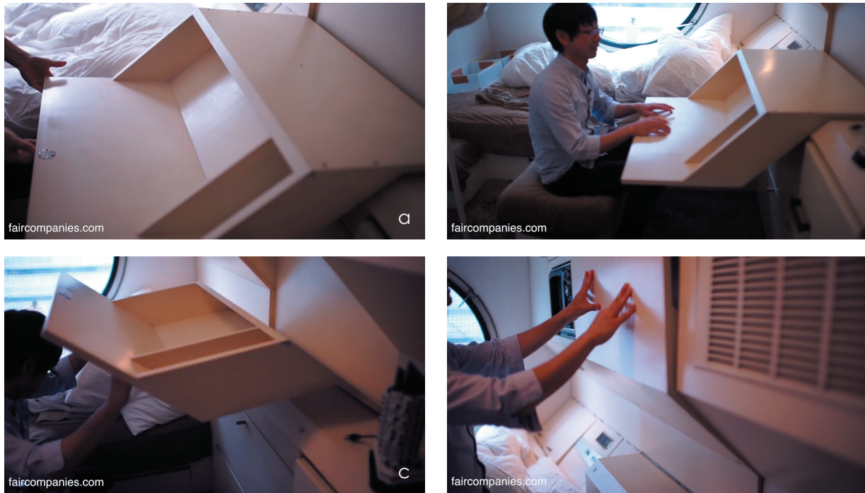
Figure 4-24(a-d). The fold-able desk in the capsule unit (Dirksen, 2015)
