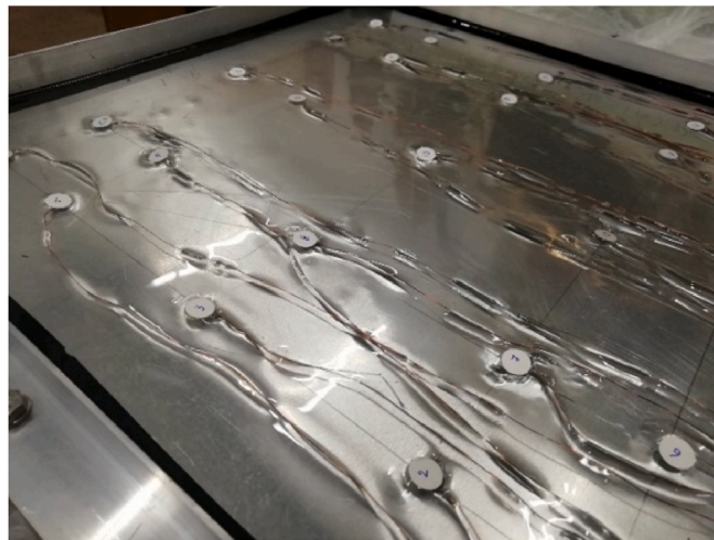
Fig. 10. Placing of the PZT sensors.
