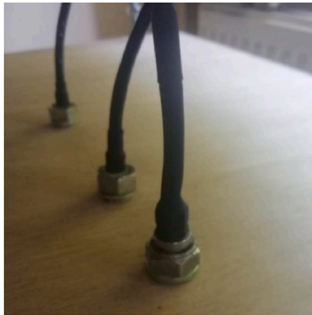
Fig. 19. Three XPM10 bolted to the mounting plate.
