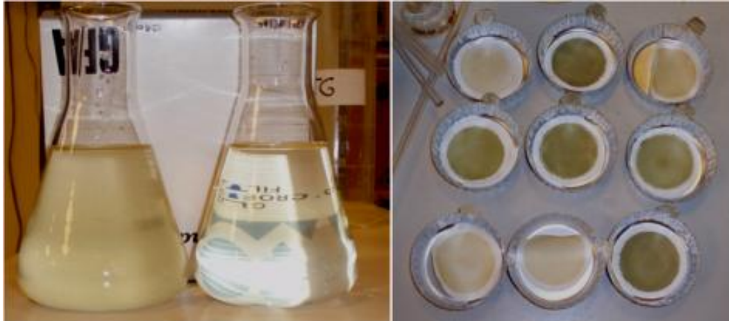
Figure 5.14 Pronounced difference between influent and effluent water (left) and filter residue.
