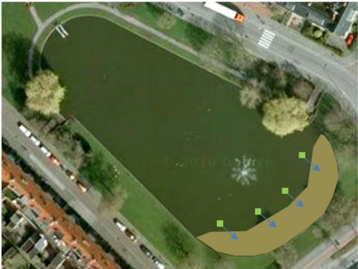
Figure 5.23 A possible combination of biofilters and a shallow zone in the Floresvijver.
