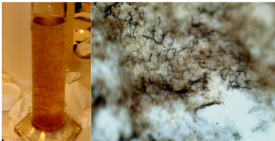
Figure 5.15 Accumulated matter from the effluent hose.
