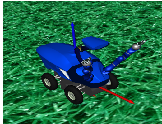
Fig. 29. Print screen of the SPANviewer GUI showing the INTERACT model and the scene around it. The arrows show the position and orientation of the world frame.
