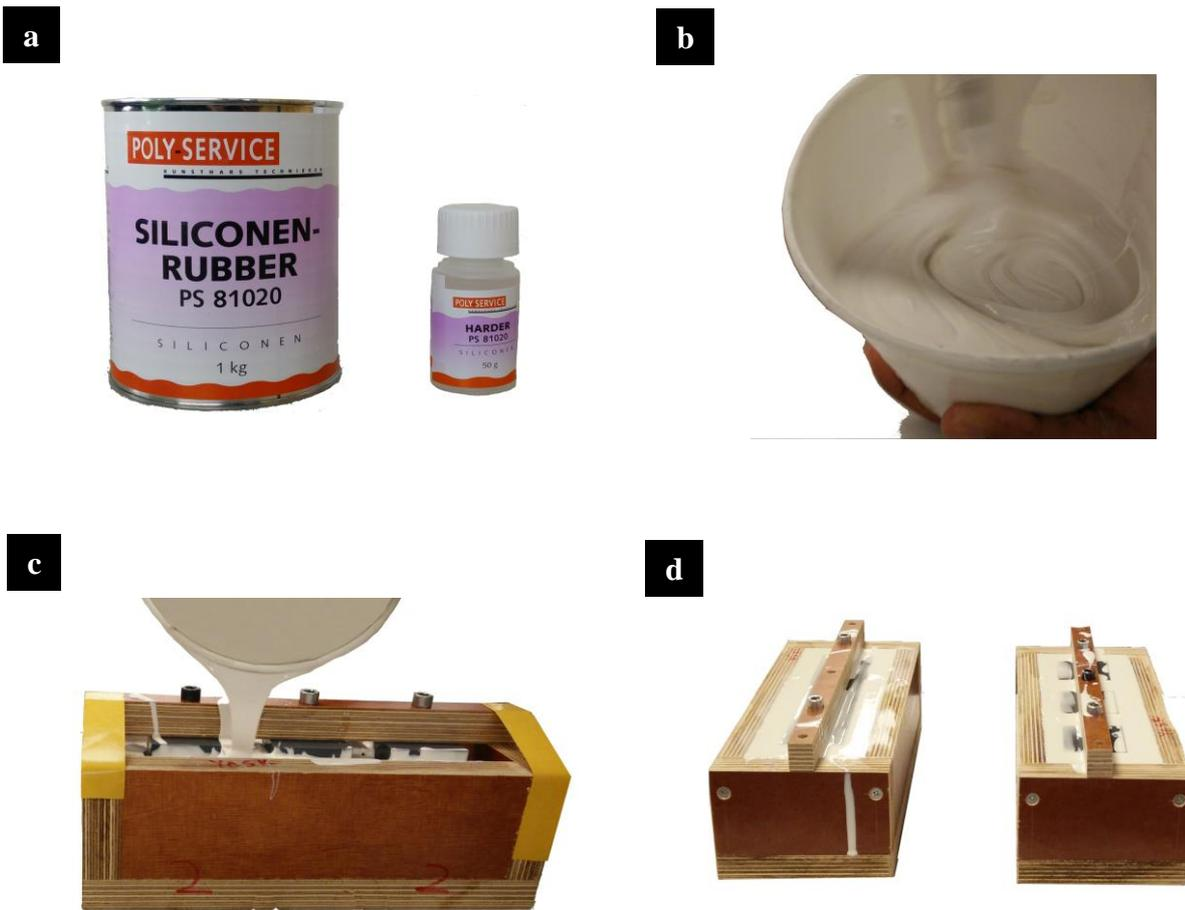
**Figure 4.2. Preparation of silicone rubber mix. (a)Silicone rubber and hardener, (b) Mixing silicone rubber and hardener, (c) Pouring silicone rubber in master mould and (d) Silicone rubber left to harden for 24h.**
