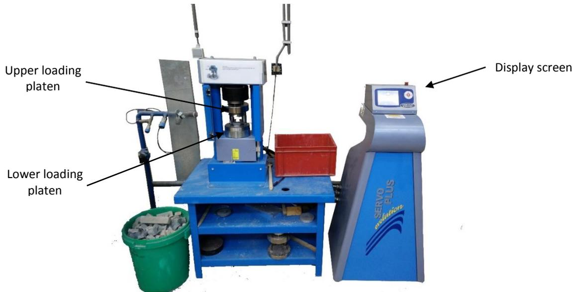
Figure 4.7. Strength testing machine generally used for concrete specimens
