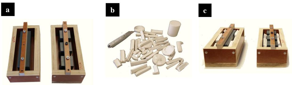
**Figure 4.1. Preparation of moulding setup. (a) Image of PVC block attached with wooden beam (225mm×15mm×17.5mm) kept in the wooden master mould. The wooden master mould consist of 5 elements: 1- 225mm×105mm×17.5mm, 2 - 225mm×15mm×17.5mm and 2 - 105mm×55mm×17.5mm, (b) Silicone rubber chopped in small pieces and (c) chunks of silicone rubber filled in the master mould.**
