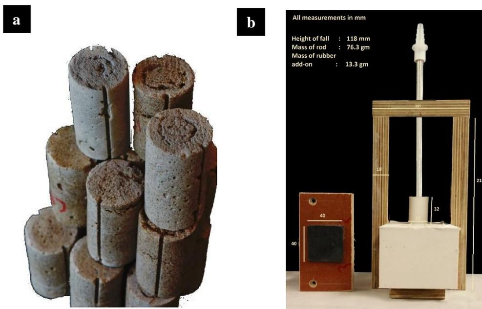
**Figure A.1. (a) Cylindrical CoRncrete specimens and (b) optimum water content setup. Optimum water content setup is helpful to indicate the optimum water content of CoRncrete. Water content where the sample shows impact activated hardness and no excess water on top, is the optimum water content.**
