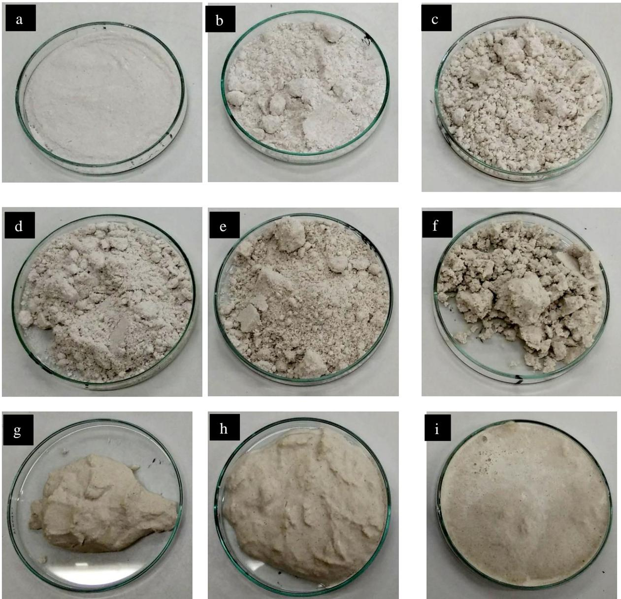
**Figure 4.10. Pictures of fresh CoRncrete (compacted with 350gm rammer) at water content (a)0%, (b)2.75%, (c)5.7%, (d)8.95%, (e)12.58%, (f)16.16%, (g)17.94%, (h)19.40% and (i)20.86%. The pictures shows fresh CoRncrete collected from the center of the sample from proctor mould for water content determination. The picture was clicked after heating the sample for 24hours in an oven at 105 °C.**
