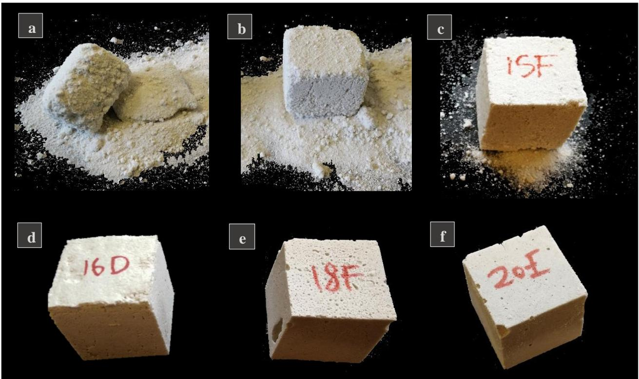
Figure 4.14. CoRncrete specimen heated in convection oven with water content (a) 10%, (b) 13.33%, (c) 15%, (d) 16.66%, (e) 18.33% and (f) 20%.
