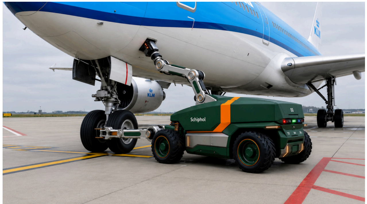
Figure 7.1: Directional visualisation of the autonomous 400 Hz connection concept for Horizon 3. Not a final technical design, but a guiding image for the workflow and requirements that follow. Image generated with the assistance of ChatGPT and Vizcom.
