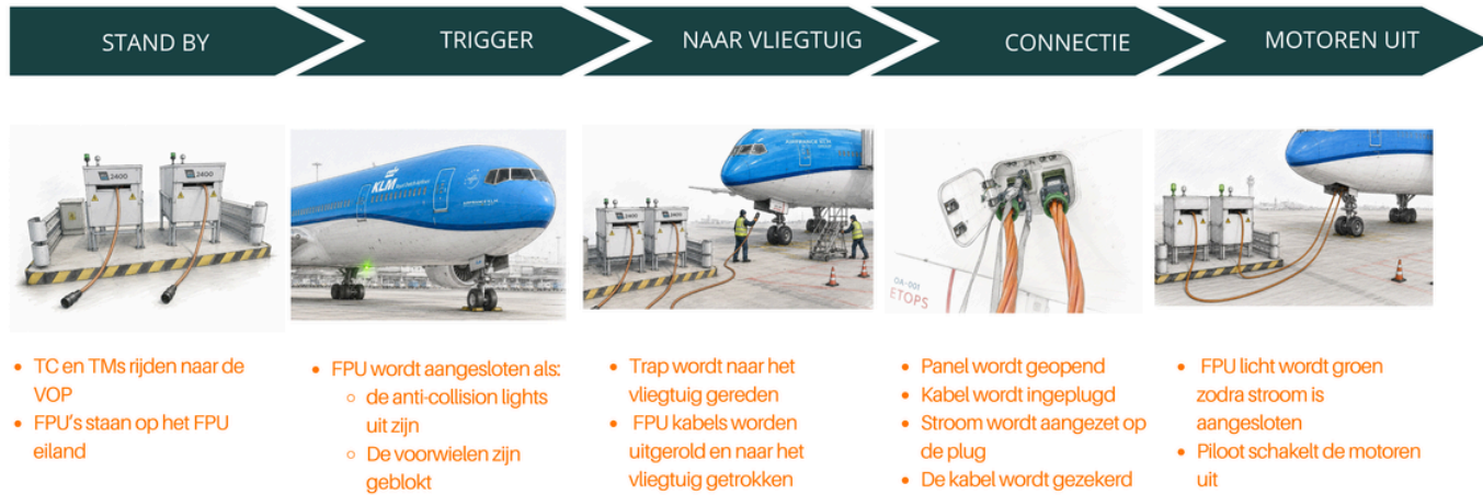
Figure I.1: Current 400 Hz connection workflow used as input for the co-creation workshop. The visual was used to create a shared understanding of the existing process and to allow participants to formulate problems. Image generated with the assistance of ChatGPT.
