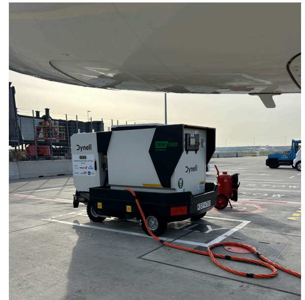
Figure 2.6: Electric ground power configurations at Schiphol: standing FPU on island (left), an FPU mounted underneath the PBB at the A-pier (centre), and a mobile e-GPU (right)
