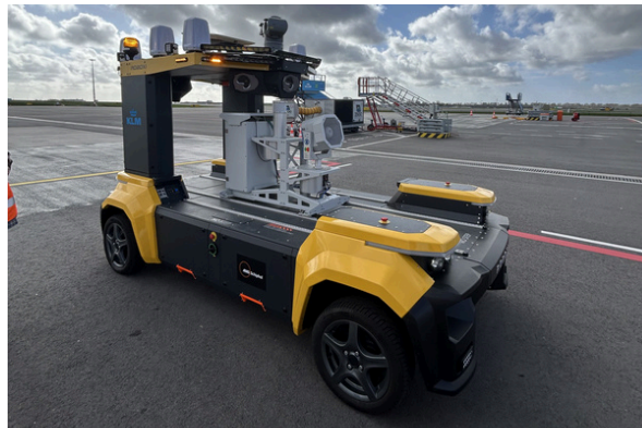
(a) Automated Foreign Object Debris (FOD) detection and removal
