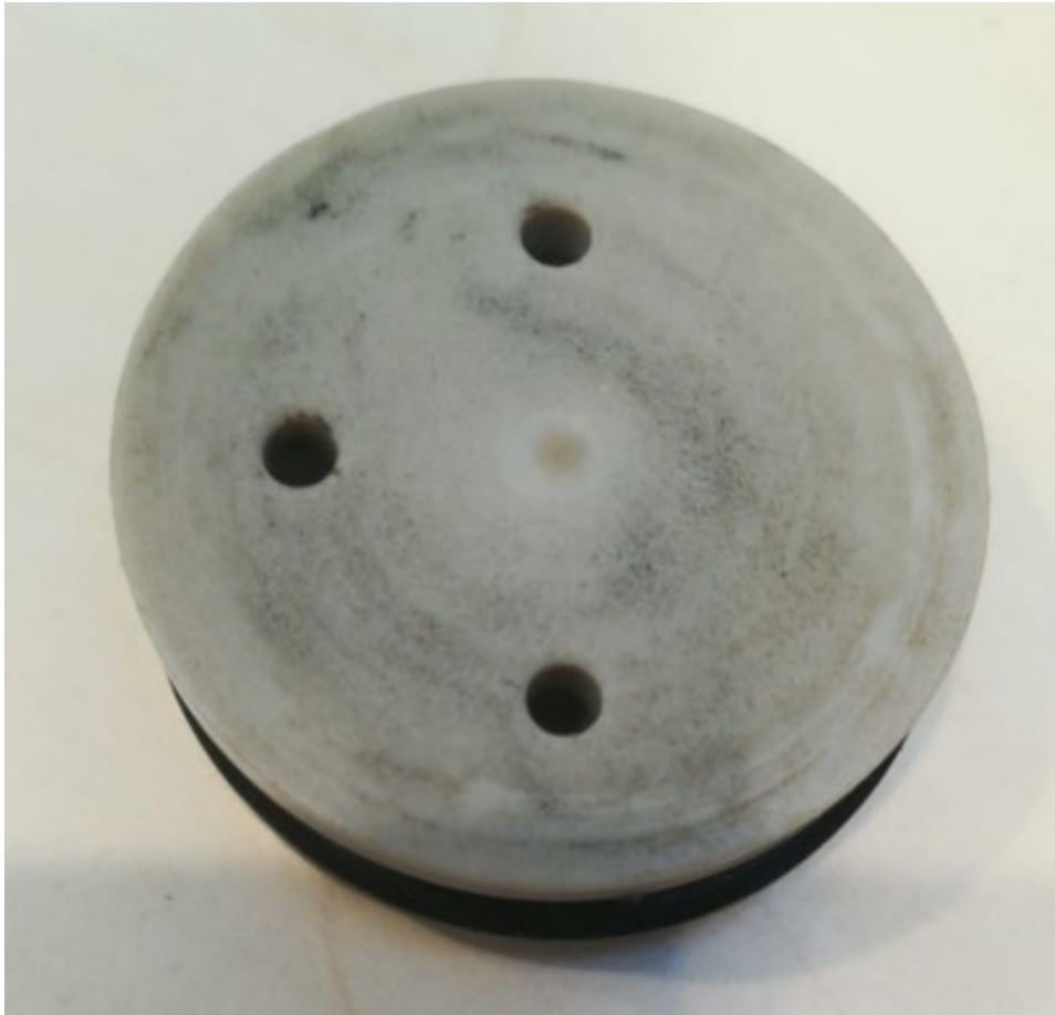
Figure A.7: The piston after an operation test
