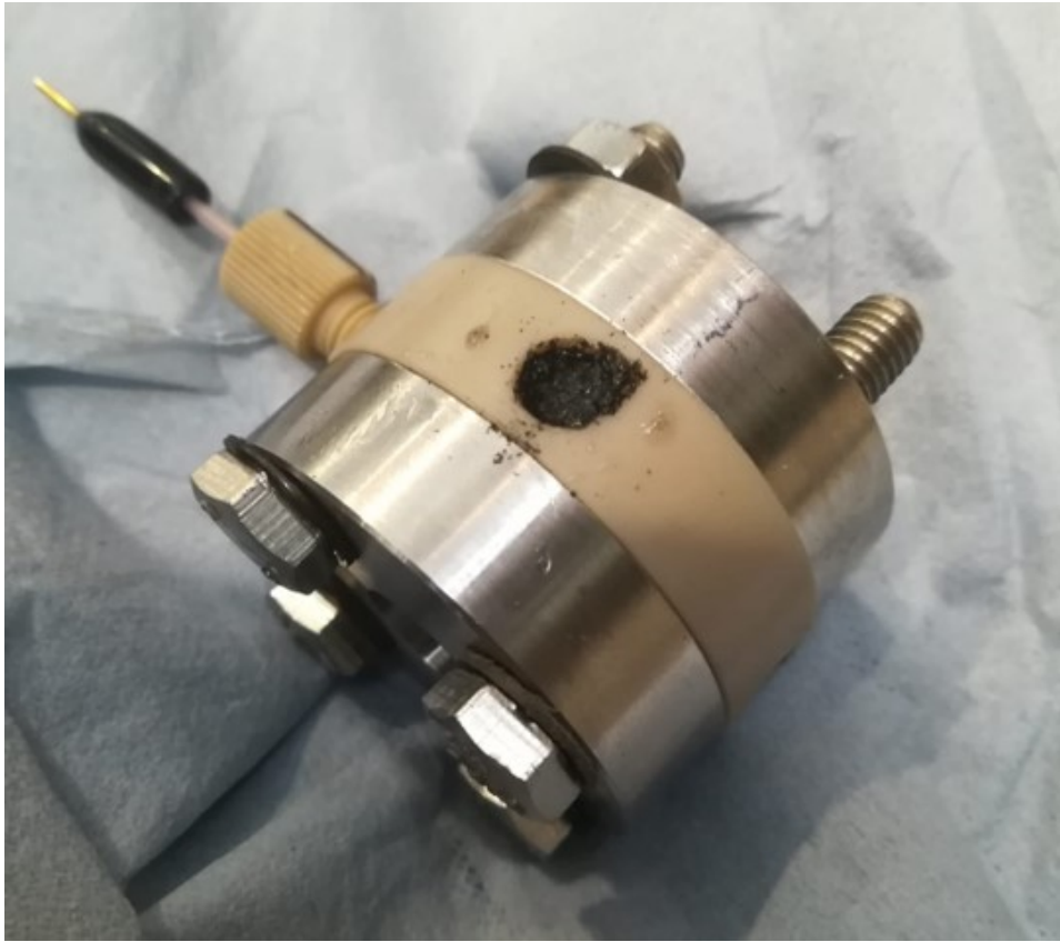
Figure A.10: reactor stack after the operation test with reference electrode.
