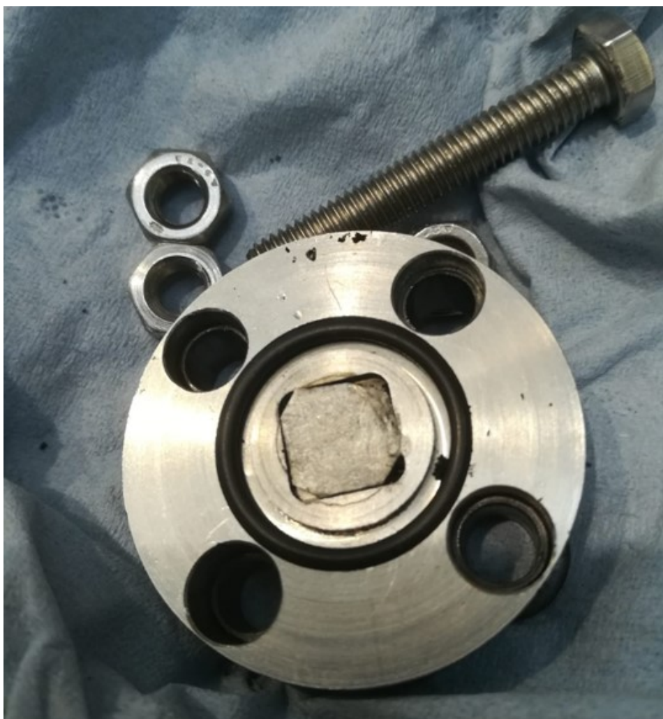
Figure A.1: The reactor casing with tin electrode and O-ring after operation.
