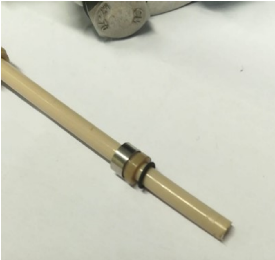
Figure A.15: Tubing with a ferrule and an O-ring.
