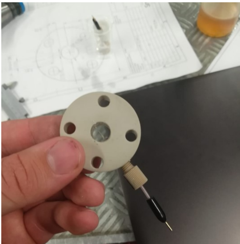
Figure A.3: Reactor chamber with added reference electrode.
