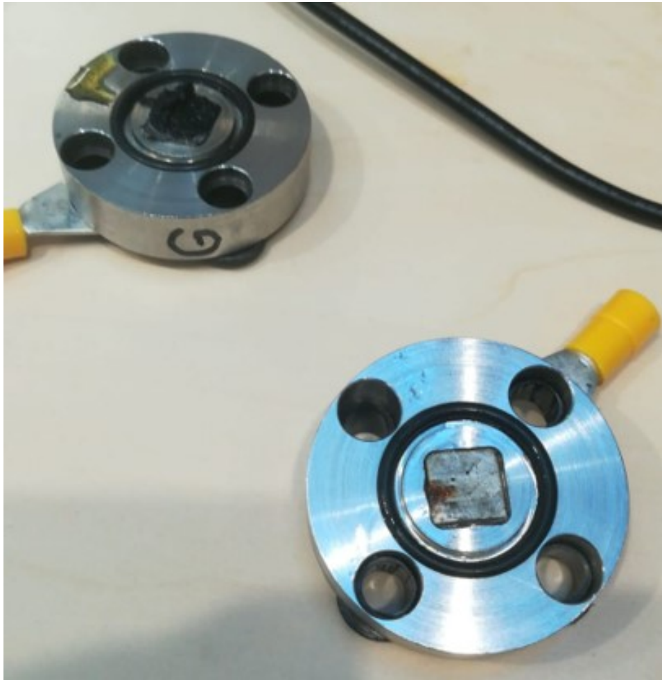
Figure A.16: The electrode casings after the operation test without reference electrode.
