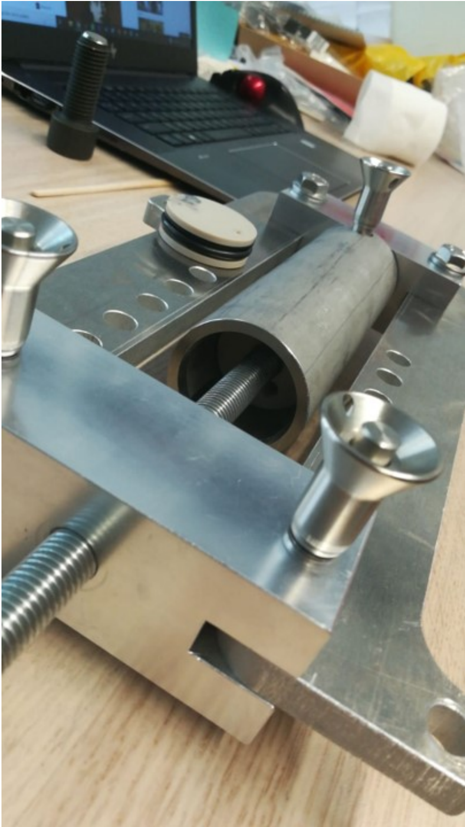
Figure A.12: The reservoir in its frame with the modified piston on top.
