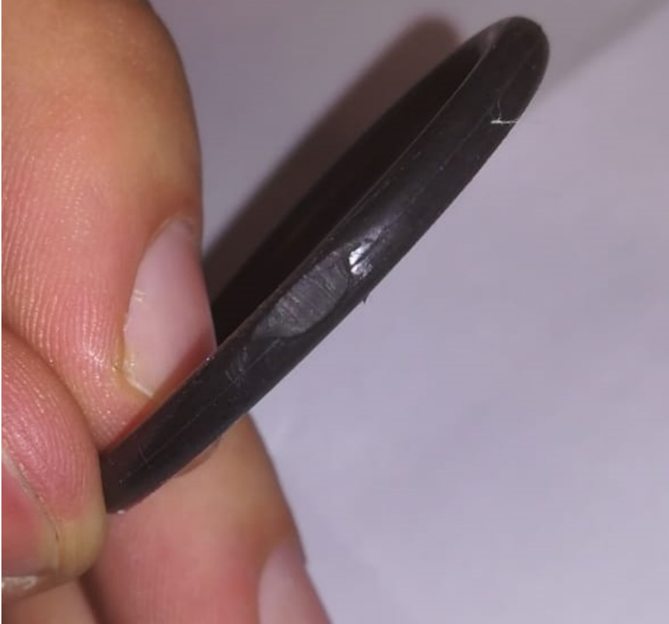
Figure A.17: A damaged O-ring
