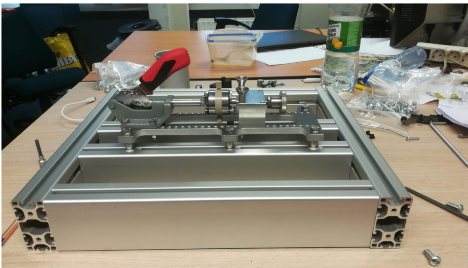
Figure A.9: The reactor stack system mounted on the bottom of the mainframe.
