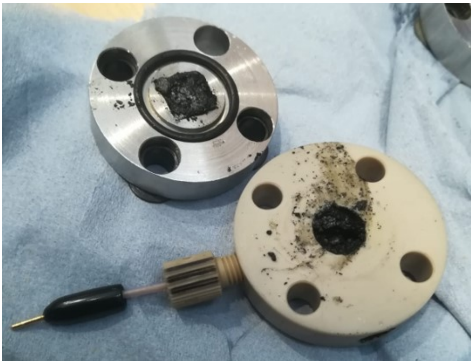
Figure A.5: Disassembled reactor stack after the operation test with reference electrode.
