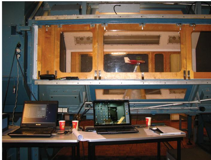
Figure 5.1: Wind tunnel measurement setup.
