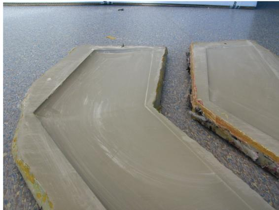
**Figure 5.11:** Wing, upper and lower surface, production molds in the process of being prepared for production.
