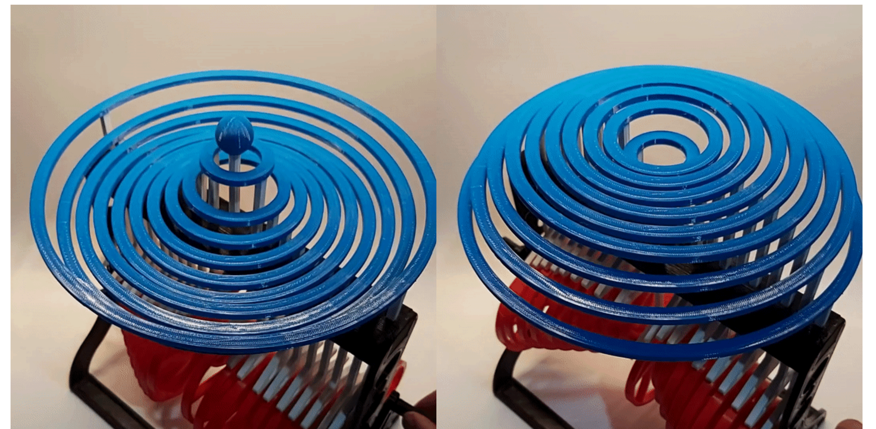
Fig. 62: Hand-cranked, 3D printed, ripple mechanism ( K4tana, 2023 )
