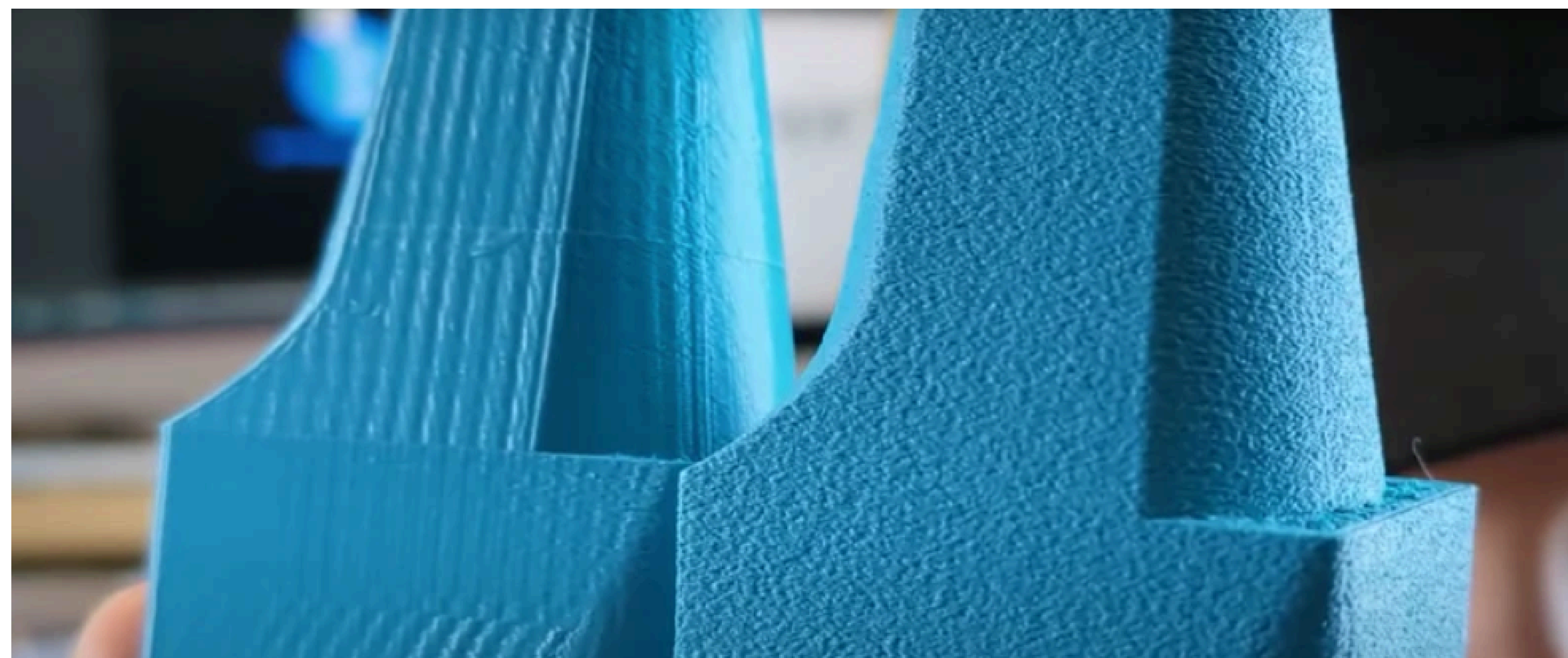
Fig. 83: Comparison between normal and fuzzy texture (Print, 2024)
