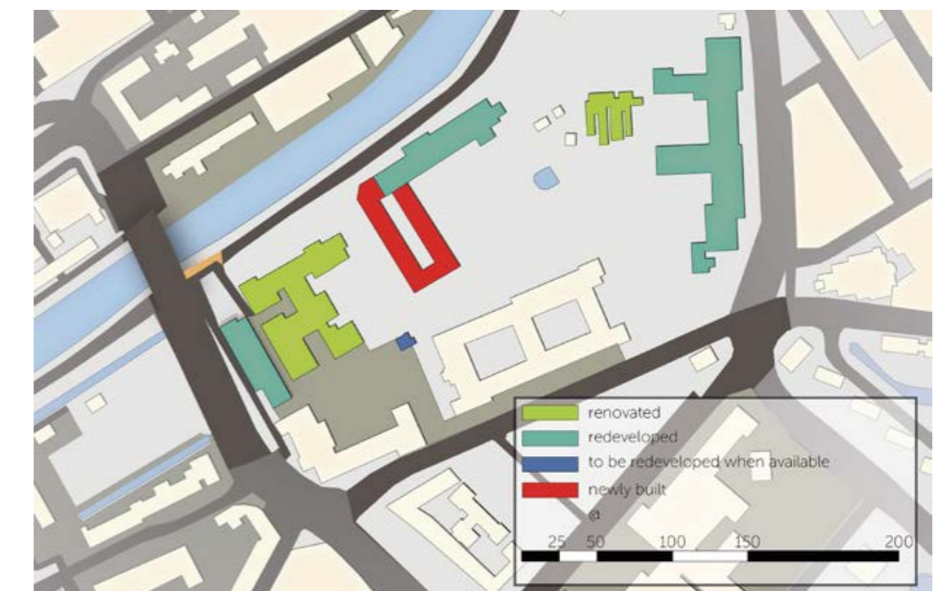
Figure 85 Renovation or redevelopment of buildings
