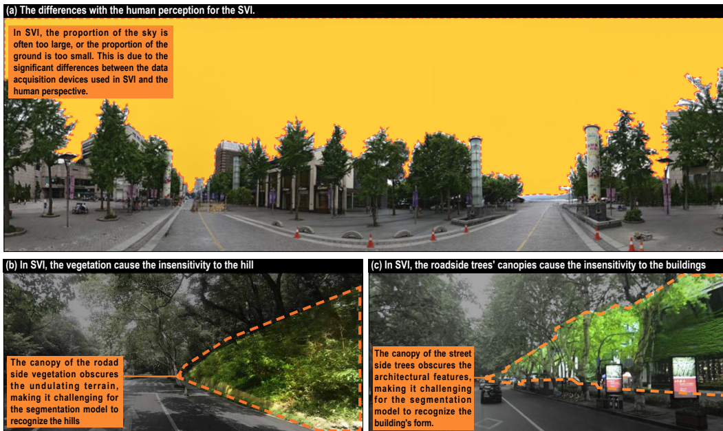
FIG. 6.10 The limitations of SVI-based methods: (a) The SVI can be far different from human perception; (b) an example of a junction node choosing preference; (c) trees block the buildings.
