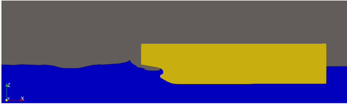
Figure 5.4: A snapshot of the ComFLOW results at t = 72.6s . The wave is starting to break and moves into the positive z-direction.
