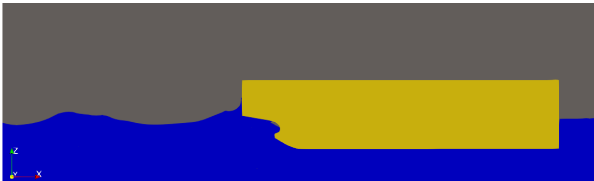
Figure 5.5: A snapshot of the ComFLOW results at t = 73.6s . The wave hits the stern flat and the energy is contained beneath the stern. This causes severe pressure pulses.
