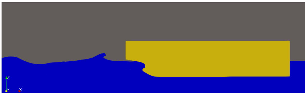
Figure 5.1: The start of a cluster at t = 67.2s event where a breaking wave leads to a big slamming event.
