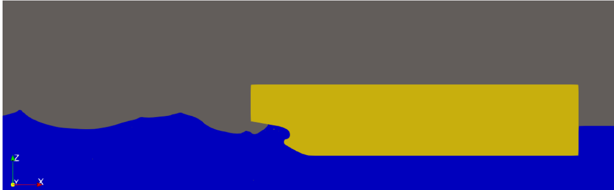
Figure 5.3: A snapshot of the ComFLOW results at t = 71.4s where the next wave moves towards the stern of the vessel. Water is sucked from underneath the stern.
