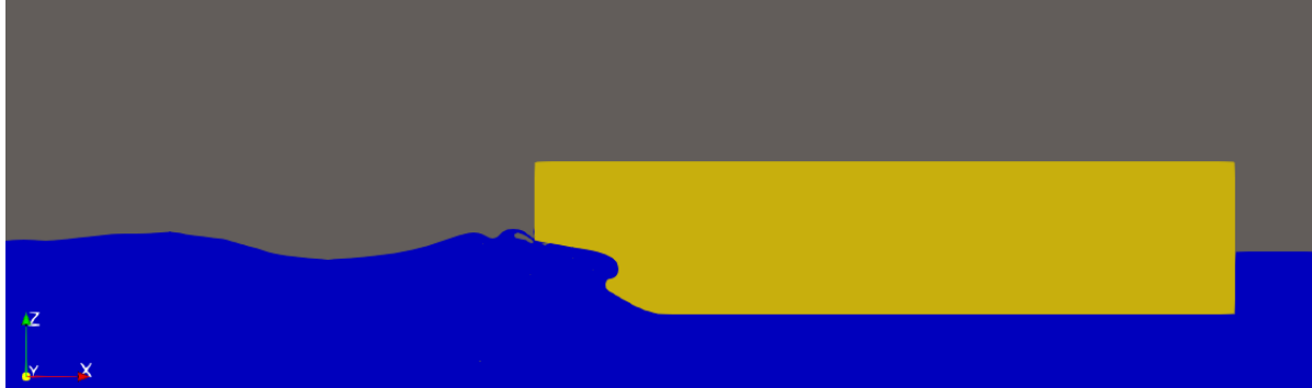
Figure 5.2: At t = 68.2s the wave reaches the stern. It creates a small pressure pulse, but most energy is dissipated by the breaking wave event.
