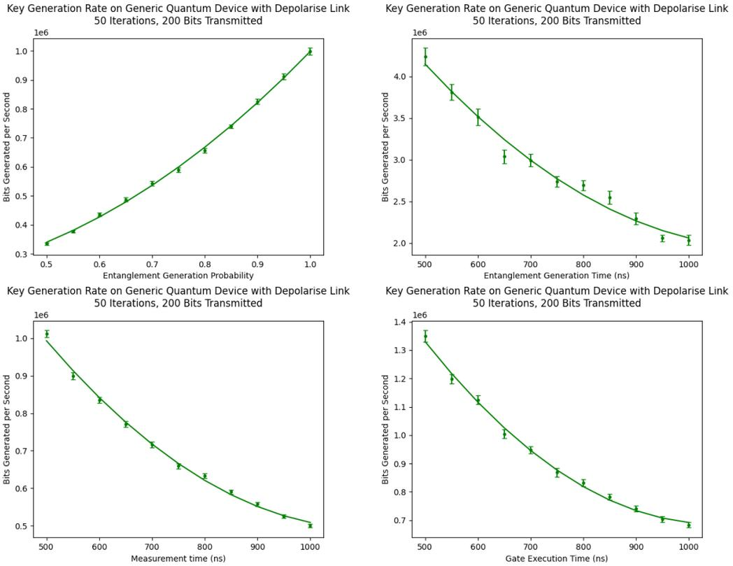
Figure 3: Key generation rate on a generic quantum device with a depolarise link
