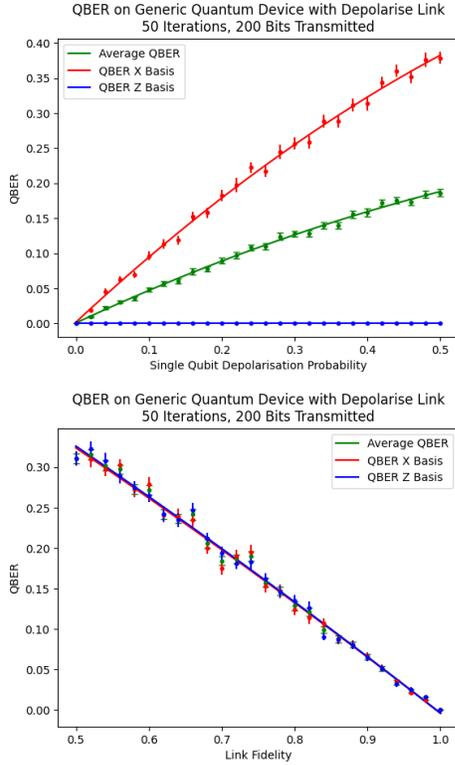
Figure 2: Qubit error rate on a generic quantum device with a depolarise link
