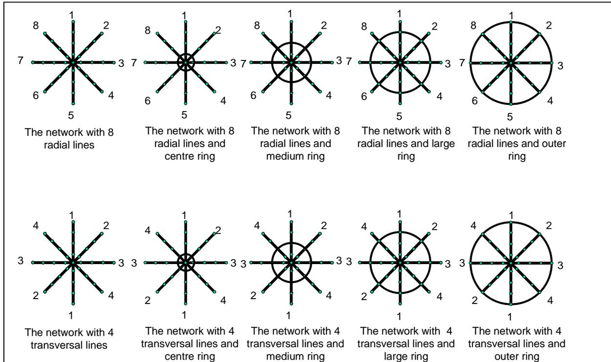
**Figure 7-2: Schematic illustration of the infrastructure alternatives in the experiments**
