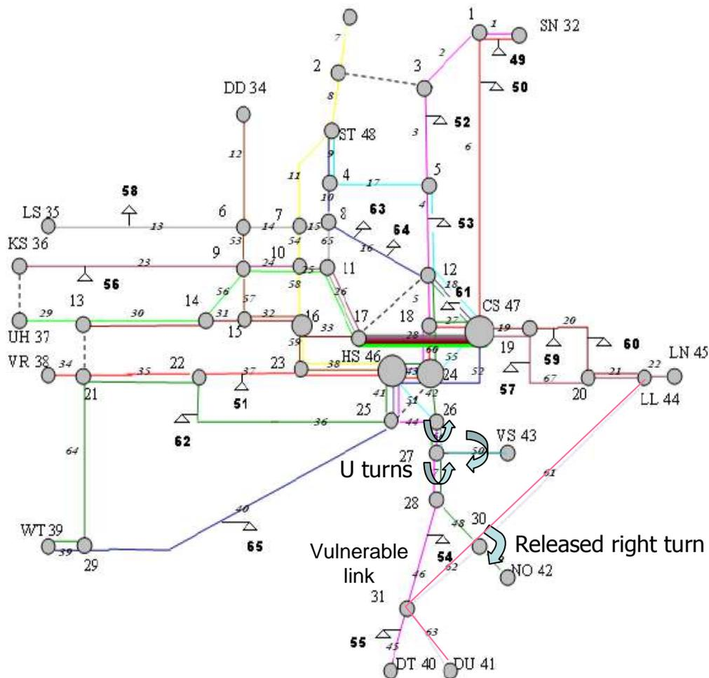
**Figure 9-10: Turning facility locations in line 1 of The Hague tram network**
