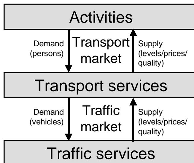
Figure 2-1: Layer model of the transportation system
