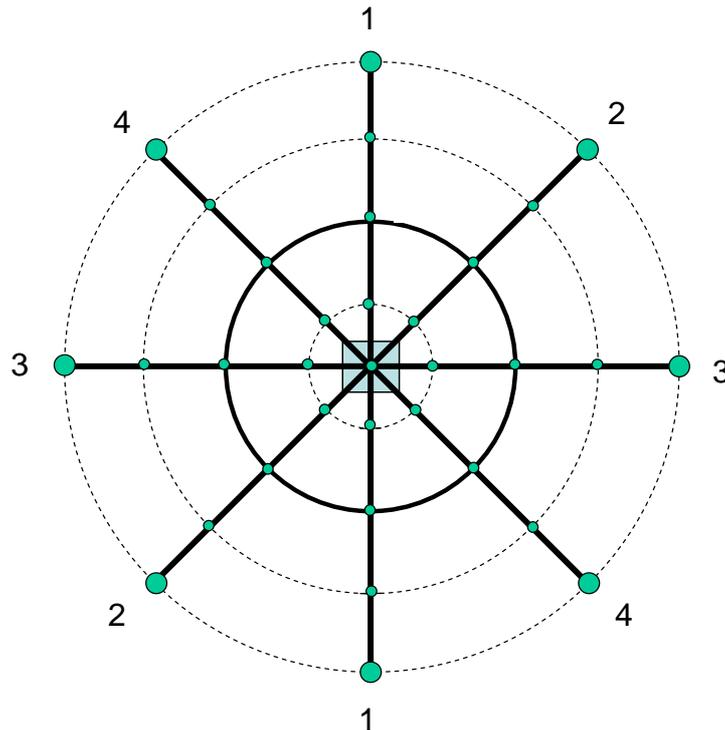
**Figure 7-9: Lay-out of the infrastructure network for variant 3: transversal line and medium ring (Line number indicated; dashed lines indicate the infrastructure for the other variants)**
