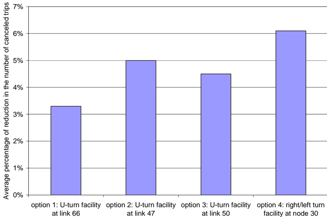
**Figure 9-11: Impacts of turning facilities on connectivity reliability of The Hague tram network**
