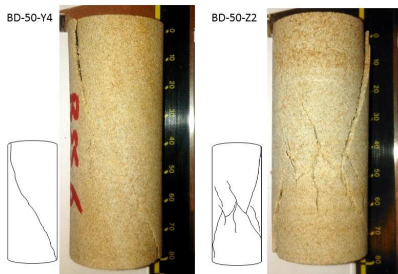
Figure 5.3: Samples BD-50-Y4 and BD-50-Z2 after the uniaxial compression test.
