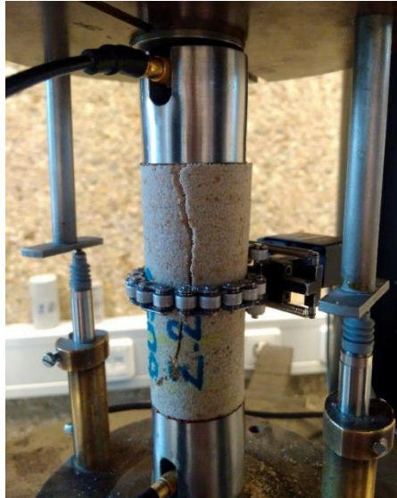
Figure 3.3: Sample BD-53-Z2B after failure from the unconfined compression test of. The sample is placed between two steel cups, in which the acoustic transducers sit in. The chain around the sample is from the extensometer, to the right and left are the LVDT's.
