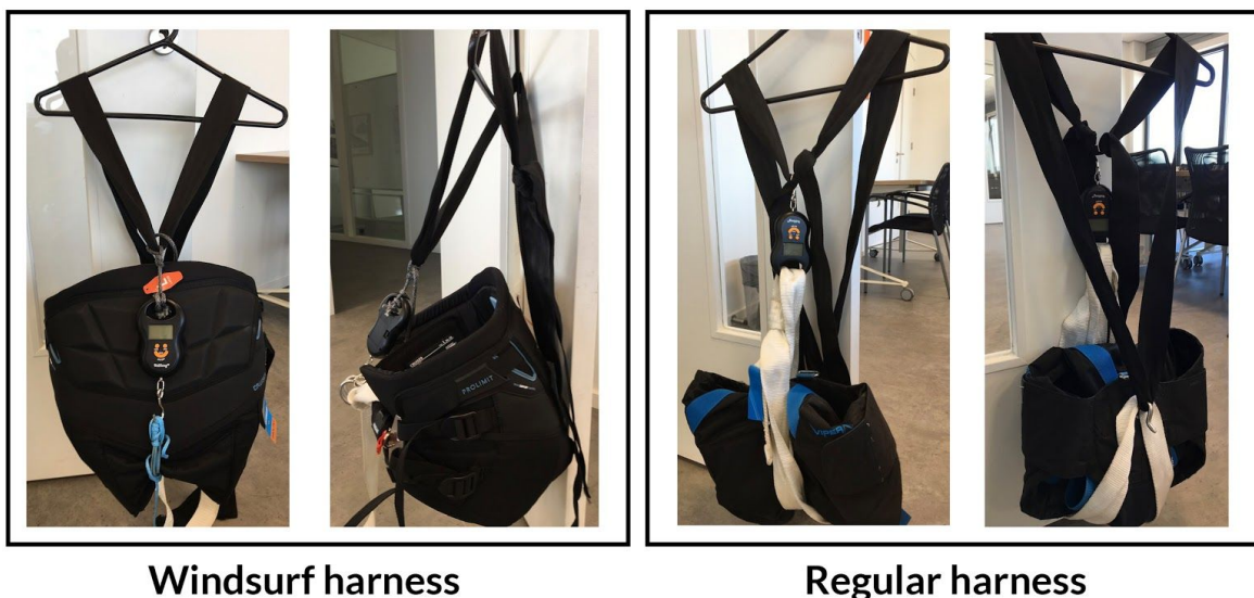
Figure [xx]; Harnesses used for the experiment with the constructed shoulder straps, left the windsurf harness and right the regular harness.
