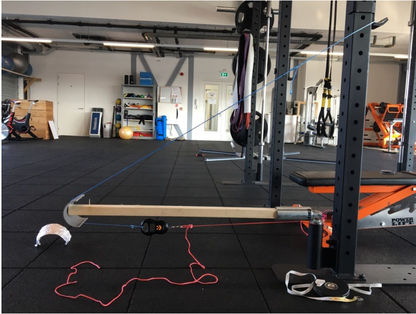
Figure A4-01; Experiment setup with the load sensor measuring F_{s2}
