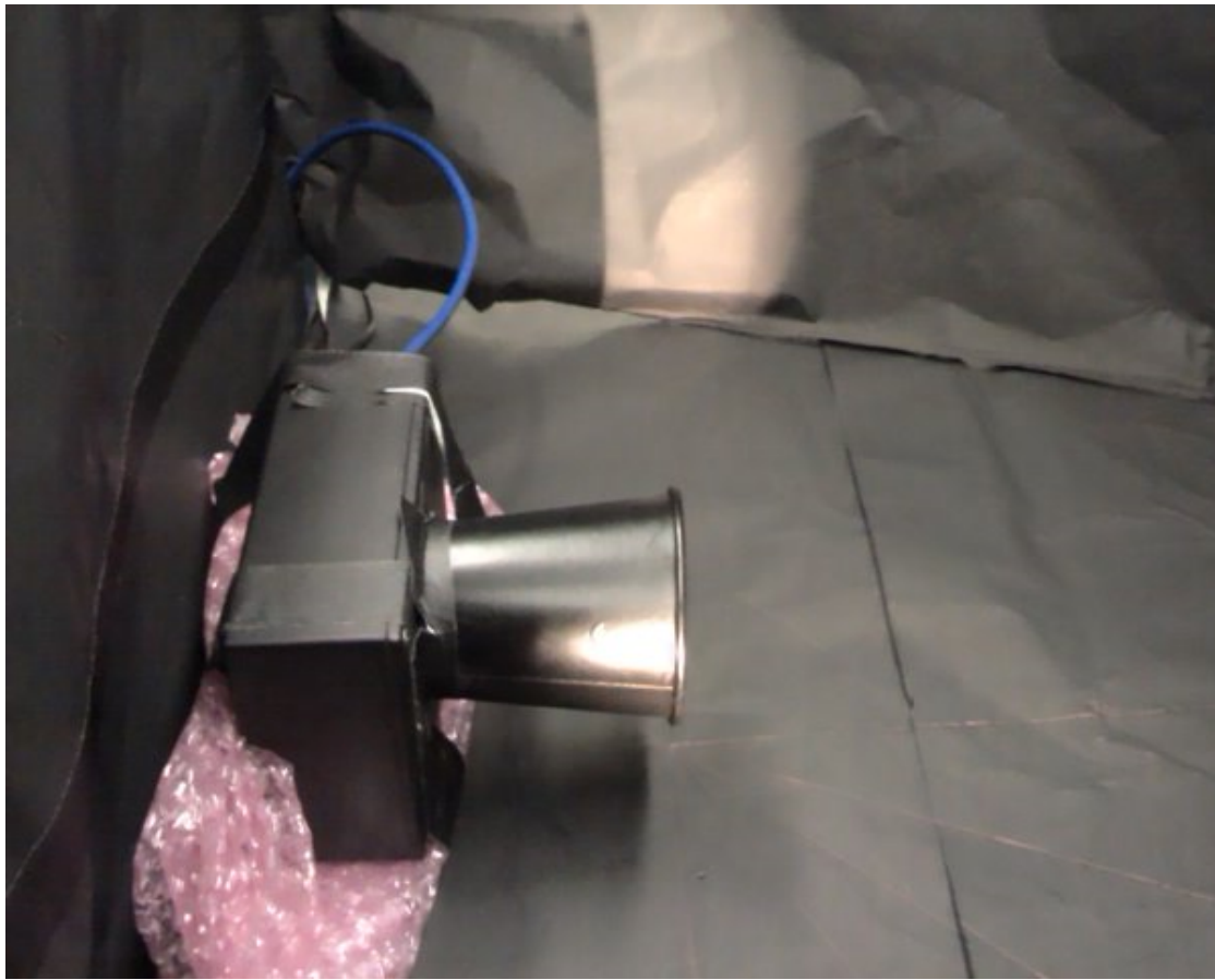
Figure 7.7: Facet Nano baffle and development mode, surrounded by black aluminum foil to absorb reflections
