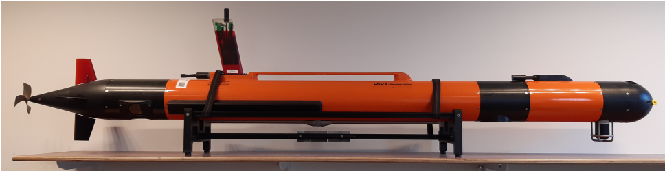
Figure 1.3.: Lightweight Autonomous Underwater Vehicle of OceanScan-MST.
