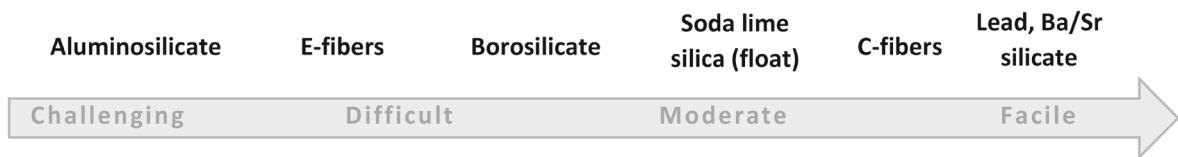
Fig. 22 Recycling by kiln-casting ease based on the chemical composition of the tested glasses
