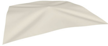
Fig. 5.34 Deformed surface from the benchmark presented in Fig. 5.33. The result is the last solution from the adaptive meshing routine with deformation norm goal functional of which the results are presented in Fig. 5.35
