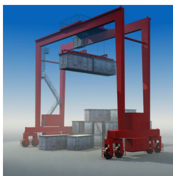
(e) RTG crane
