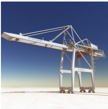
(a) STS crane
