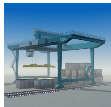
(f) RMG crane
