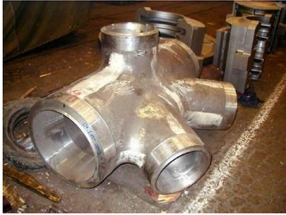
**Figure 8.7: Cast steel joint [6]**
