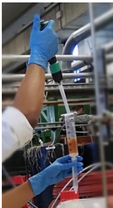
Figure 5 Passing of samples from Multilayer sand filtration through resin for Arsenic Speciation
