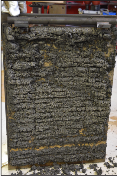
Closed element with the burned and expanded fire retardant coating after the measurement. At some places there is no burned coating because it fell of when we put wet towels on the element in order to prevent further smoke production.
