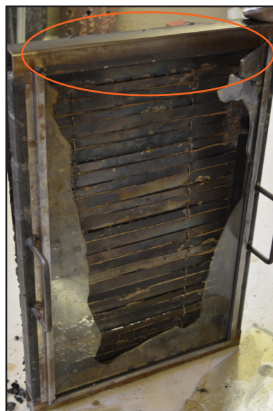
4 mm glass with the closed element at 75 mm distance and a fire retardant coating. Breakage at 102.5 degrees Celsius.
