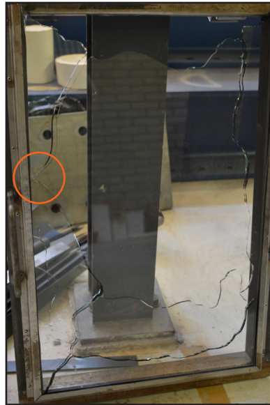
6 mm glass with the open element at 75 mm distance. Breakage at 99.1 degrees Celsius.
