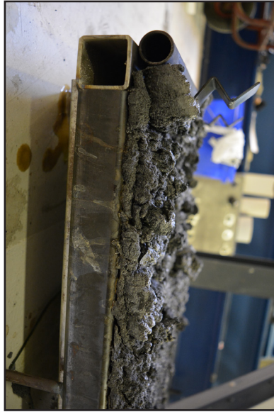
Photo of the expanded fire retardant coating. The coating has expanded from 0.7-1.0 mm to 2-3 centimetres.
