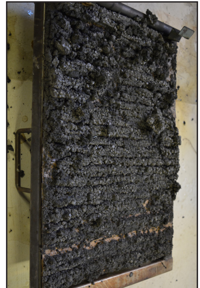
Photo of the expanded fire retardant coating.
