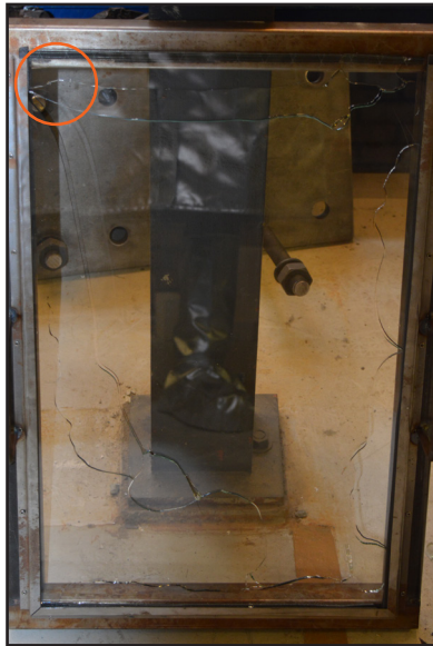
4 mm glass with the open element at 75 mm distance. Breakage at 103.8 degrees Celsius.
