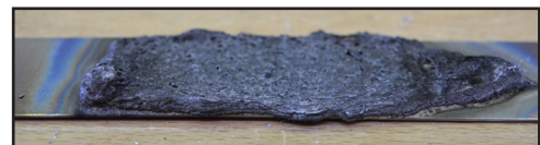
Photo 8: expanded fire coating from 0.9 (dried) mm to 3.1 - 9.0 mm
