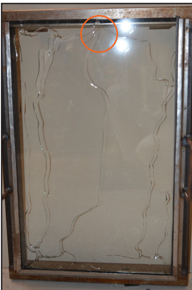
6 mm glass with the open element at 100 mm distance. Breakage at 118.7 degrees Celsius.
