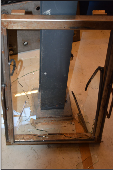
4 mm glass without an element. Breakage at 109 degrees Celsius.
