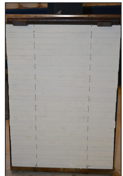
Closed element with fire retardant coating of 0.7-1.0 mm thick. Before the measurement.
