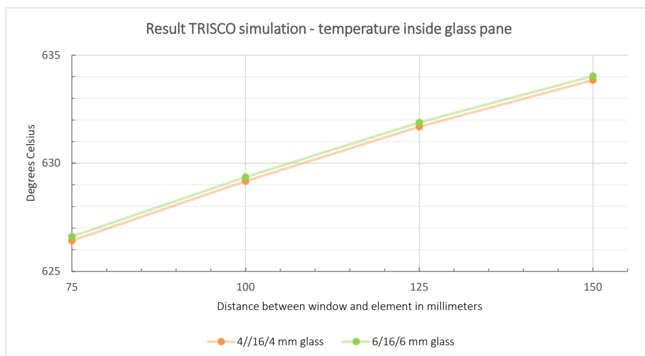
Graph 6: result of the TRISCO simulation with the different types of glass
