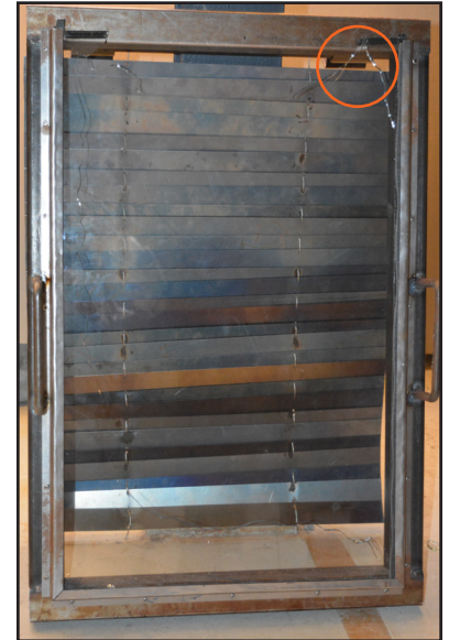
4 mm glass with the closed element at 75 mm distance. Breakage at 70.0 degrees Celsius.
