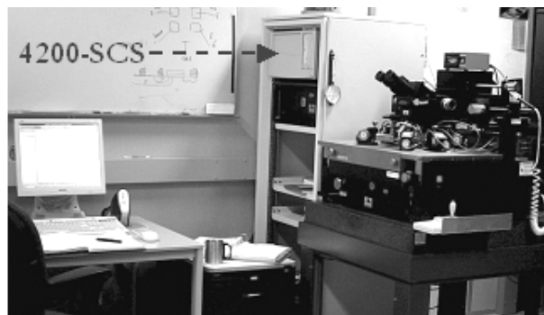
Figure 3.3 A Keithley 4200-SCS in the mismatch characterisation system.
