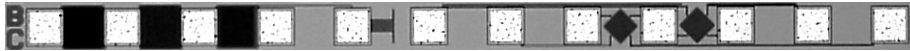
Figure 2.4 Example of a 1xM pad frame module for a scribe line test structure.
