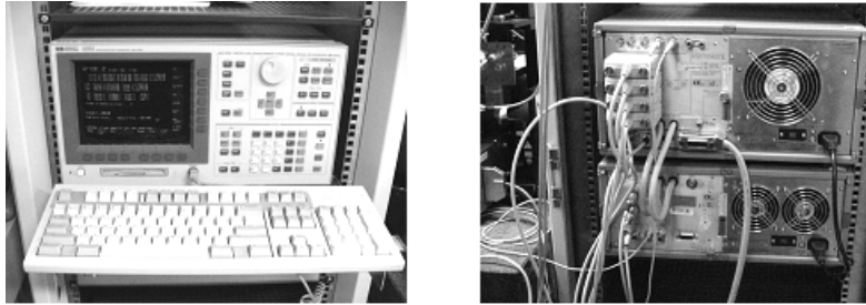
Figure 3.2 The 4156 front panel and back plane (including 41501 expander) with double triaxial cabling for the HRSMU's.
