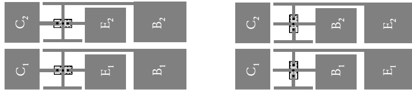
Figure 2.28 Two implementations of matched pair that consist of two individually padded (discrete) transistors.
