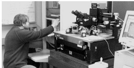
Figure 3.1 At work with the HP4156/CM 12k mismatch measurement system.
